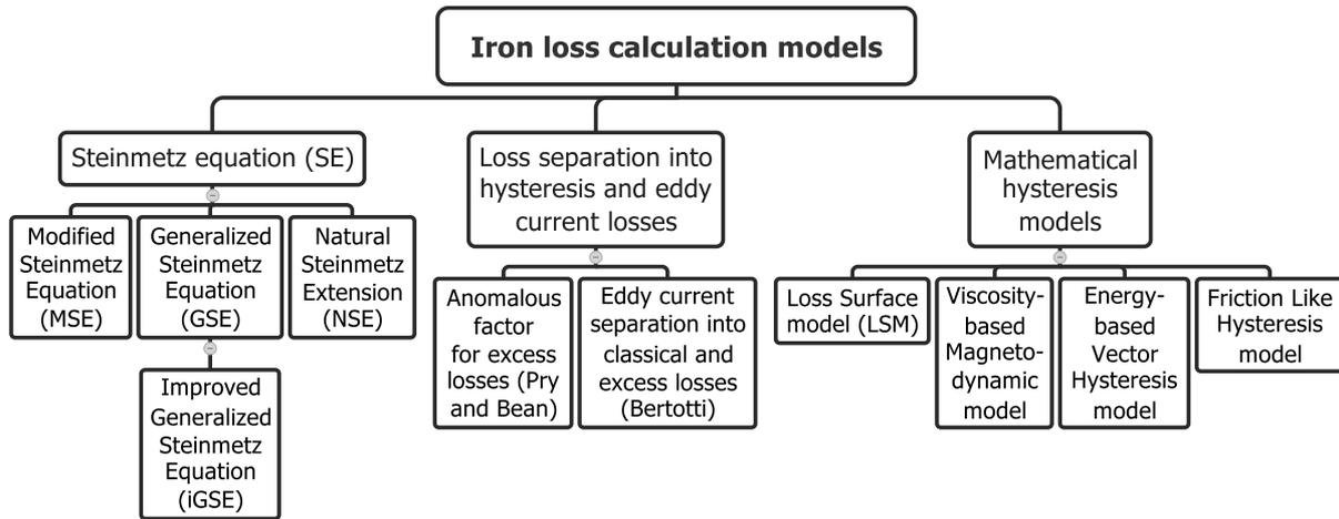
Figure 1: Model approaches to determine iron losses in electrical machines.
