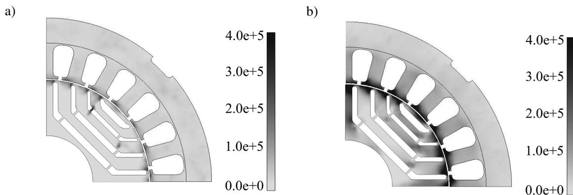
Figure 7: Resulting iron loss density distributions ( $\text{W/m}^3$ ): a) 1500 rpm, 108 Nm; b) 3000 rpm, 72 Nm.
