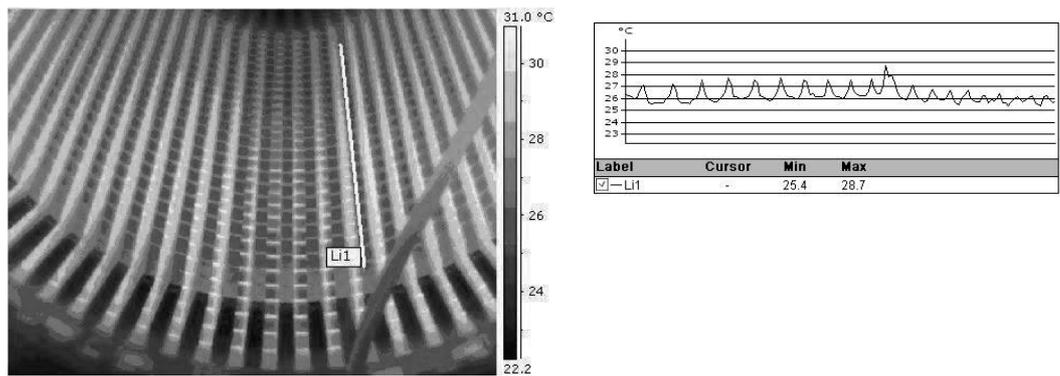
(a) Thermal image of a stator during core-flux test. (b) Temperature along line Li1 shown in 13a
