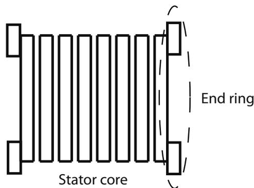
Figure 10: Location of the end rings at the stator core made of lamination packages and separated by cooling ducts.
