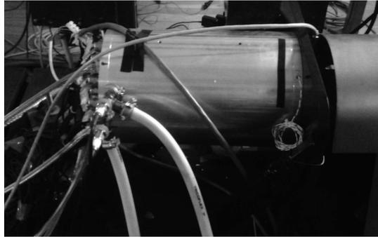
Figure 6: Experimental setup. The front hoses carry inlet and outlet water for the water jacket.
