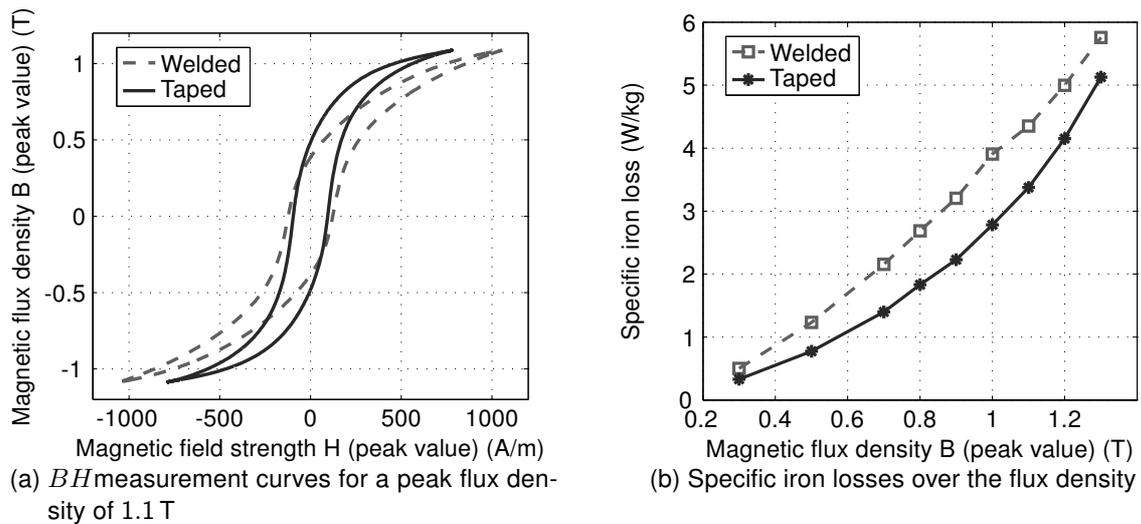
Figure 9: Measurement results of the welded and taped ring cores at 50 Hz.
