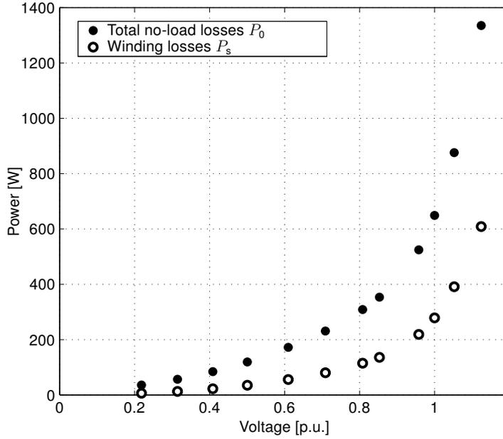
Figure 3: Measured no-load losses at rated frequency as a function of voltage.
