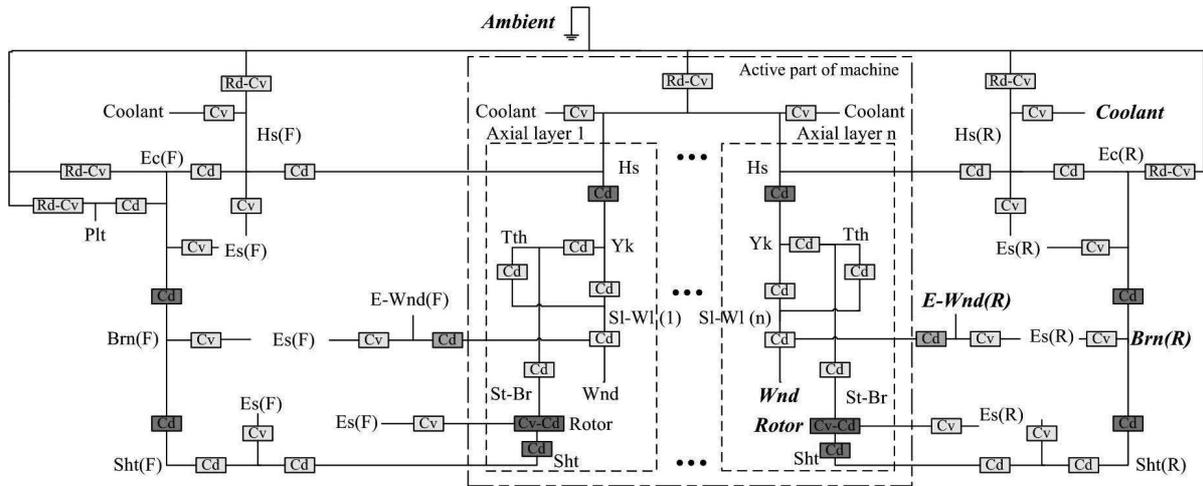
Figure 5: Complete LP thermal model of the PMSRM. The abbreviations used are reported in Table 1. Loss sources are indicated as dots. The bold highlighted words also represent temperature sensor locations in the experimental setup.
