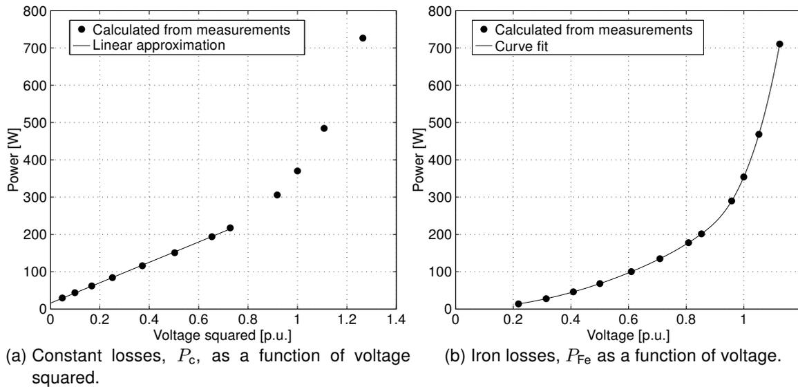
Figure 4: Determination of friction and windage losses (a) and iron losses (b) from measurements.
