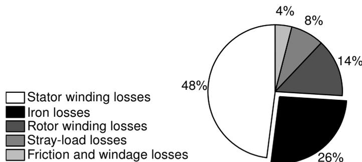
Figure 2: Distribution of the total losses at rated power for the studied 11 kW induction machine.
