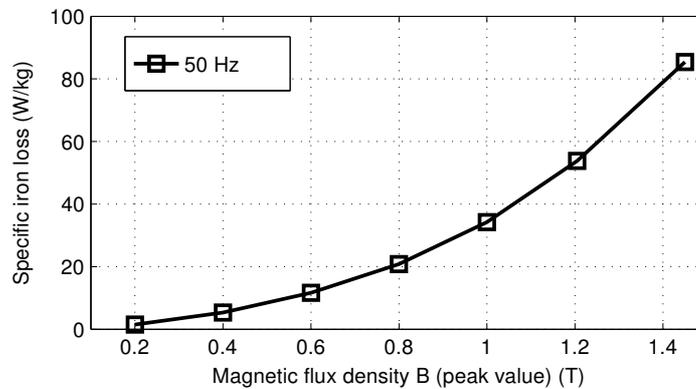
Figure 12: Measured iron loss at different flux densities.
