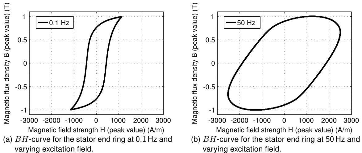
Figure 11:  $BH$ -curves for the solid test sample representing the stator end ring.
