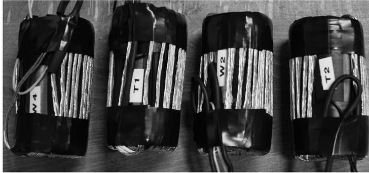
Figure 8: Wound stator ring cores for magnetic measurements.
