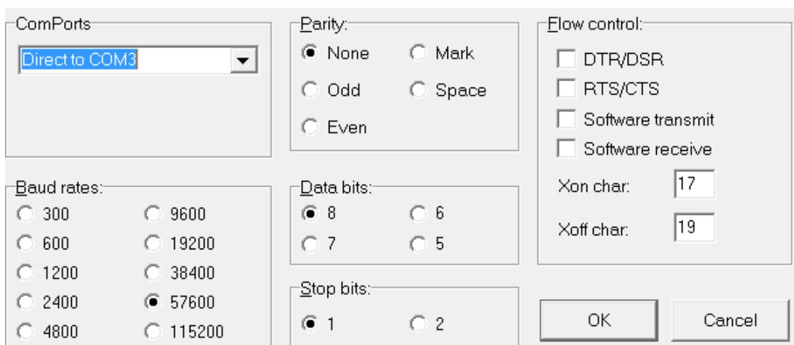
Figure 3.10 Set up of S6350 RFID Reader
