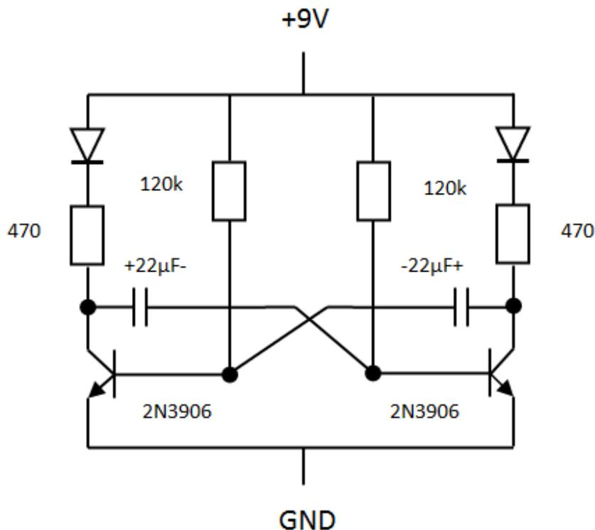
Figure 3.16 Blinking LED circuit
