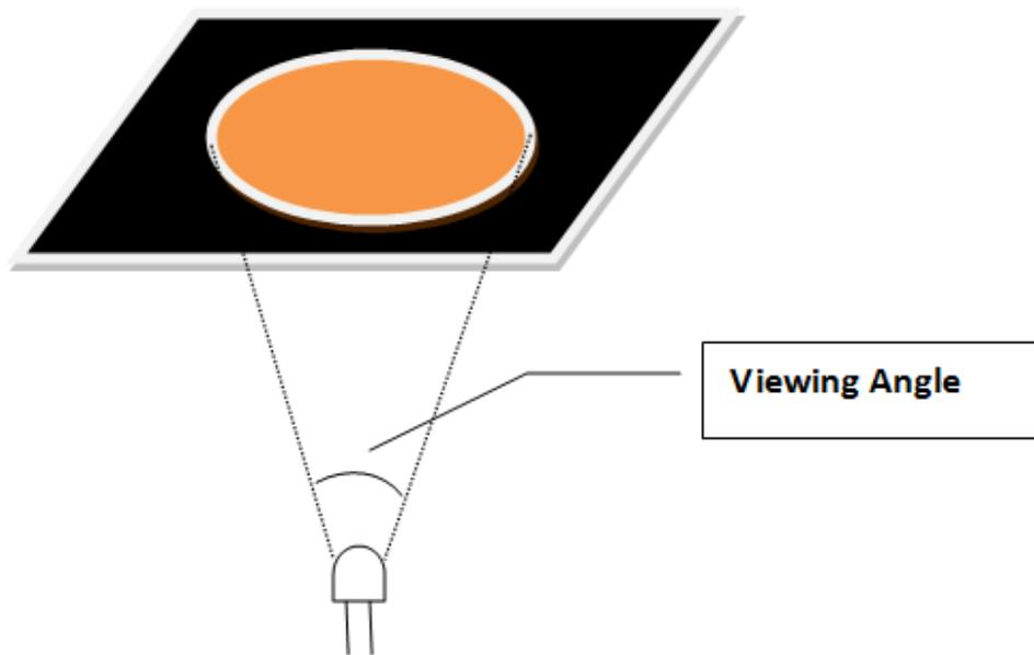
Figure 3.15 View Angle of standard LEDs
