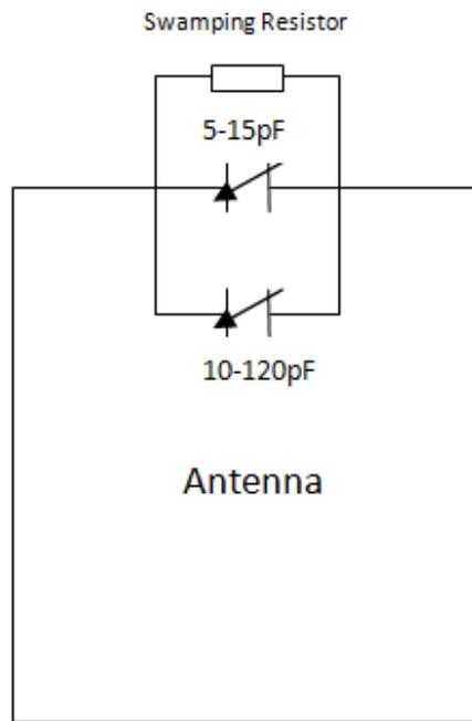
Figure 3.8 The resonant circuit on the antenna
