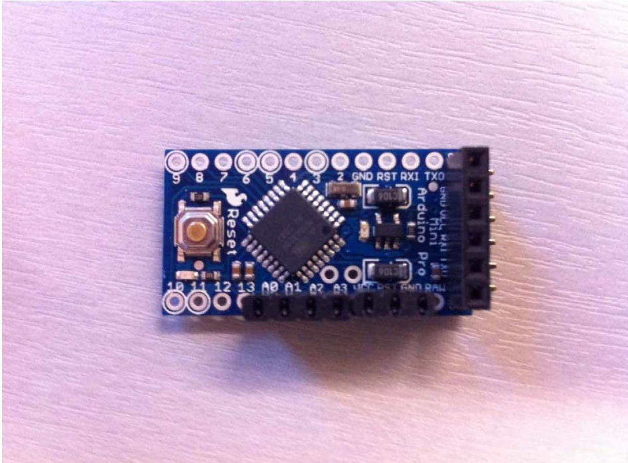
Figure 3.1 Arduino Pro Mini
