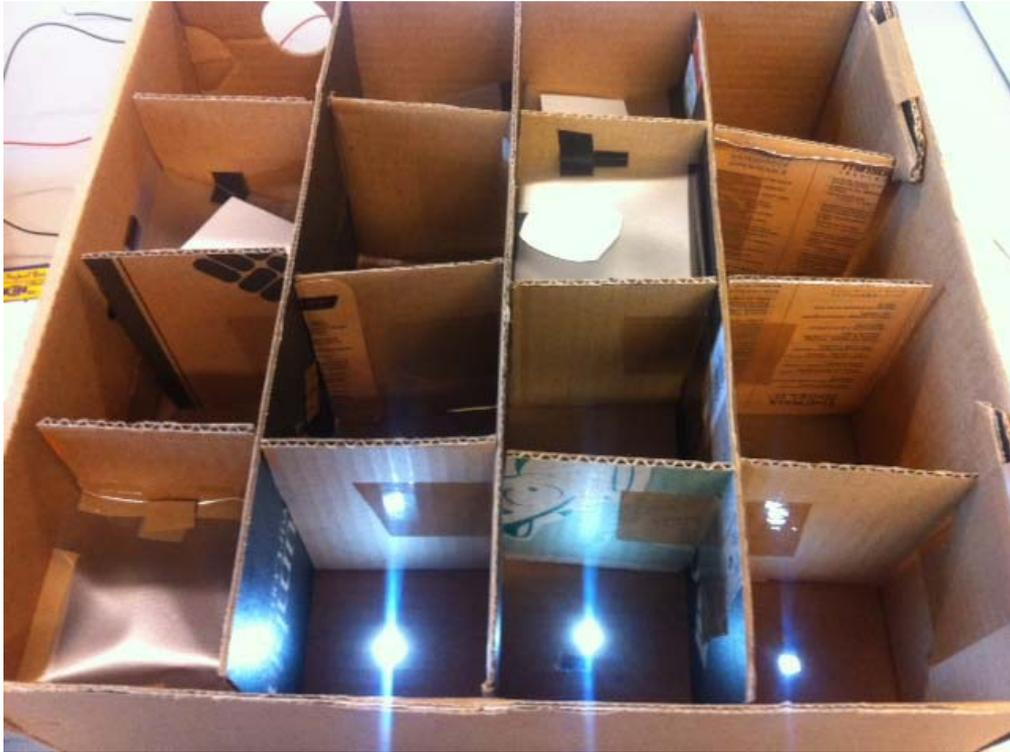
Figure 3.13 Activation box with high performance LEDs
