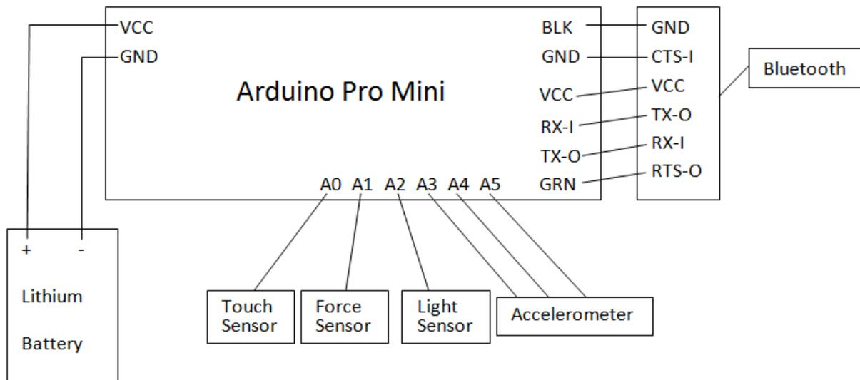
Figure 3.6 The overview of the components of SEI-E Object
