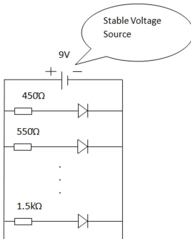
Figure 3.12 Circuit for controlling LED's luminous intensity
