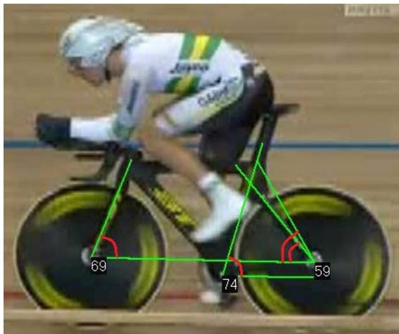
points in the center of the rear hub. The angles lie between the wheel-base axis and the longitudinal axis of the seat stay (bike geometry) resp. the axis from rear hub to the center of the top end of the seat tube (common geometry). The latter seat tube angle is the more important angle in this analysis. The Top Tube angle (slope of the top tube; not in the picture) can be neglected because it is horizontal at the bikes of the five athletes.
