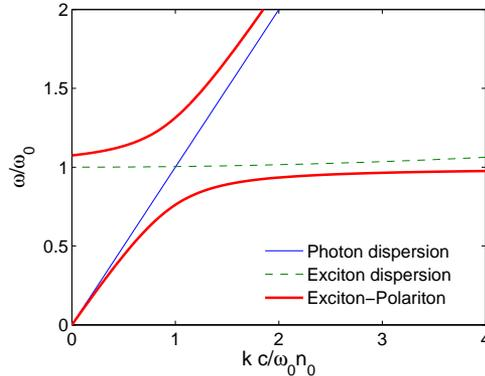
Figure 3.2: The dispersion diagram for photons, ground-state exciton and the exciton-polariton
