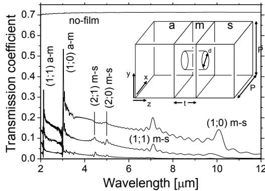
Figure 4.3: Transmission coefficient of a metal thin film with  $3 \mu\text{m}$  period  $1 \mu\text{m}$  diameter hole array calculated by FDTD. Inset: schematic geometric grating structure. Plasmon  $(i;j)$  modes are labelled, "a-m" and "m-s" denote air-metal and metal-semiconductor interfaces. From low to high transmission curves:  $d = 800, 1200, 1600 \text{ nm}$ ; The curve at about 0.7 denotes the case without any metal film.
