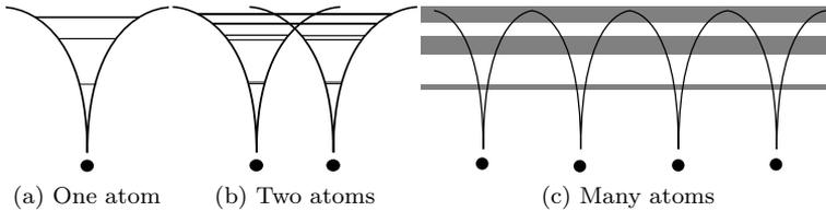
Figure 2.1: Illustration of the forming of bands
