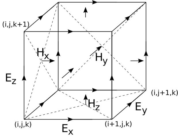
Figure 5.1: The Yee lattice, which staggers the E and H field components in space. The E components are placed at the edges and the H components are placed at face centers
