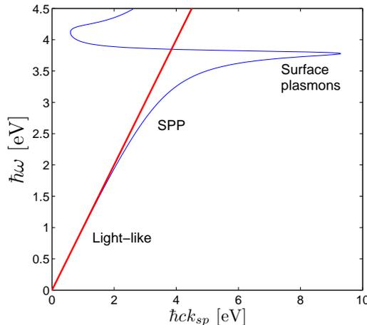
Figure 4.2: The surface plasmon polariton dispersion, using the Drude fit to silver presented in figure 4.1
