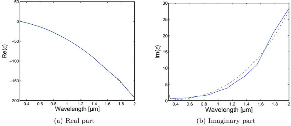
Figure 4.1: The dielectric constant of silver, measured data taken from[22], with a fit using the Drude model (dashed line)
