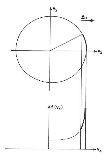
Fig.3. Illustration that the new ions retain their beam character in the direction of  $\underline{v}_0$ , even if the instability takes the time 0.5  $\omega_{\text{ci}}^{-1}$  to tap their energy.
