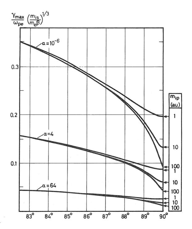
Fig.6. The growth rate for almost perpendicular propagation, where it is influenced by the plasma ion mass m<sub>ip</sub>. The growth rate at  $\theta$  =90° is expressed by Eq. (VII).
