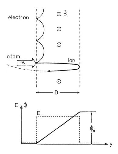
Fig. 2. The ionizing front model according to Piel et al (1980).
