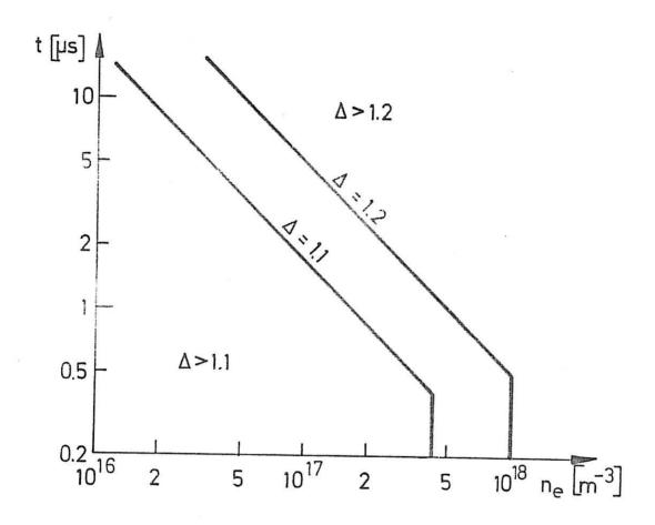
Figure 6 Uncertainty factor  $\triangle$  in the quantity  $\aleph$  in fig. 5 as a function of electron density  $n_e$  and experimental time in an idealized experiment, where the density is zero for t<0 and ne for t $\geqslant$ 0.
