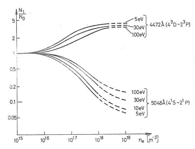
Figure 2 The effect on the intensities of two spectral lines of excitation transfer with zero imprisonment and  $T_{\rm e_1}$  between 5 and 100 eV. The results are uncertain, where the curves are dotted.
