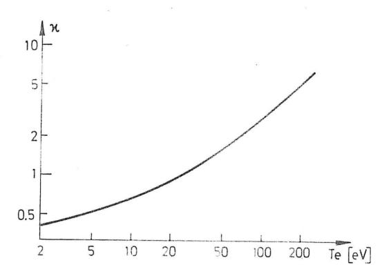
Figure 5 The relation between the quantity  $\alpha = \sqrt{N_{5048} \cdot N_{4922}}/\sqrt{K^{\circ}N_{4713}}$  and the electron temperature. K is found in fig. 3 as a function of the degree I of imprisonment.  $\alpha$  is uncertain with a factor  $\Delta$ , that can be found in fig. 5 as a function of electron density and experimental time.
