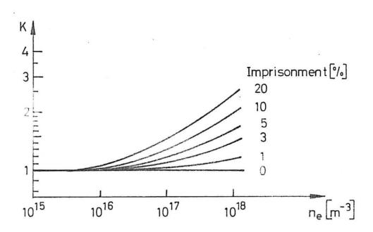
Figure 4 Factor K to be used in connection with fig. 4, as a function of electron density and degree of imprisonment I.
