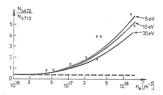
Figure 3 Intensity ratio for the two lines 4472 Å (4<sup>3</sup>D-2<sup>3</sup>P) and 4713 Å (4<sup>3</sup>S-2<sup>3</sup>P) as measured (crosses) and calculated from excitation transfer rate equations of 5, 10 and 30 eV (solid lines). Excitation from the ground state alone would give the same value (dotted line) for all electron temperatures and densities.
