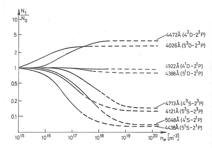
The effect on the intensities of eight spectral lines from excitation transfer at  $T_{\rm e}=10$  eV and zero imprisonment.  $N_{\rm o}$  would be the intensity if only excitation from the ground state were important.  $N_{\rm l}$  is the calculated intensity with excitation transfer considered. The results are uncertain where the curves are dotted.
