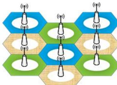
Figure5. Frequency distribution with omnidirectional antenna
