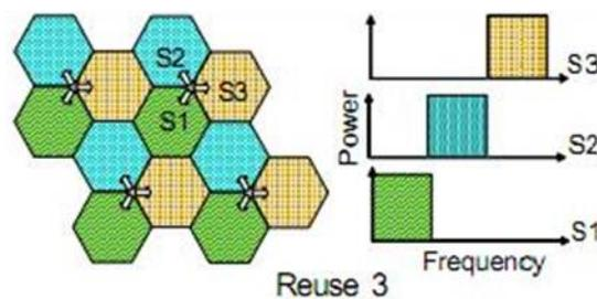
Figure2. Hard frequency reuse scheme with reuse 3 [14]
