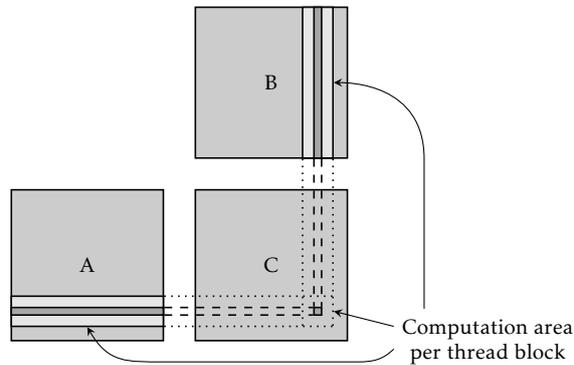
FIGURE 4.8 – Matrix multiplication using thread blocks.
