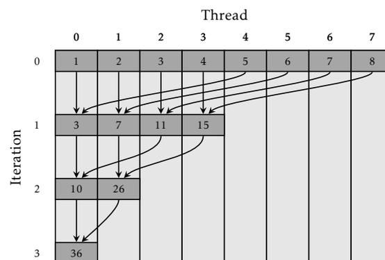
FIGURE 4.12 – Sum reduction – improved approach. Source: adapted from [32].
