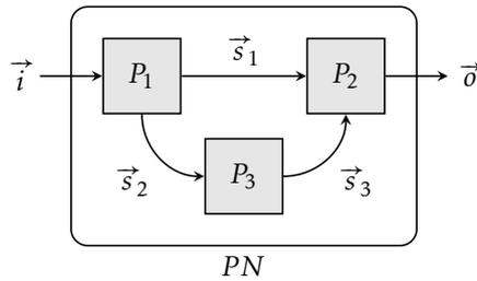
FIGURE 2.1 – Example of a ForSyDe model, which can be viewed as a network of concurrent processes. Source: adapted from [41].
