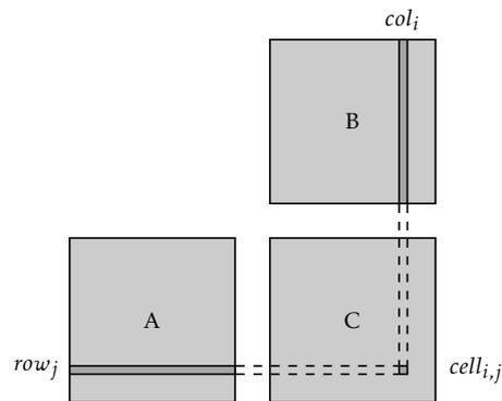
FIGURE 4.6 – Matrix multiplication. *Source: adapted from [32].*
