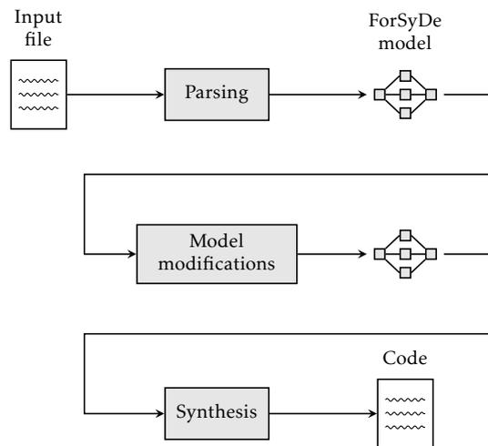
FIGURE 9.1 – Overview of the component data flow.
