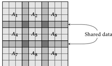
FIGURE 10.2 – A 2-dimensional input data set, where each set consists of a  $4 \times 4$  submatrix that partially overlap with its neighboring data sets.
