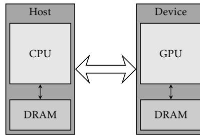
FIGURE 4.5 – Host and device separation in CUDA.
