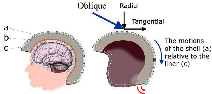
**Figure 2.** Schematic picture of the MIPS helmet, made of a hard shell (a) separated from the liner (c) by a low friction layer (b). At an oblique impact the shell can move relative to the liner.
