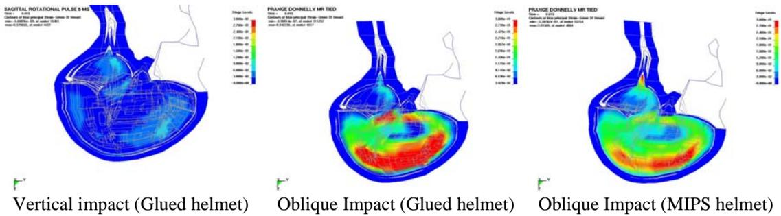
**Figure 6.** The pictures show the strain in the xy-plane 5mm offset the sagittal plane. The red colors show the regions where the strain is close to the injury thresholds for DAI.
