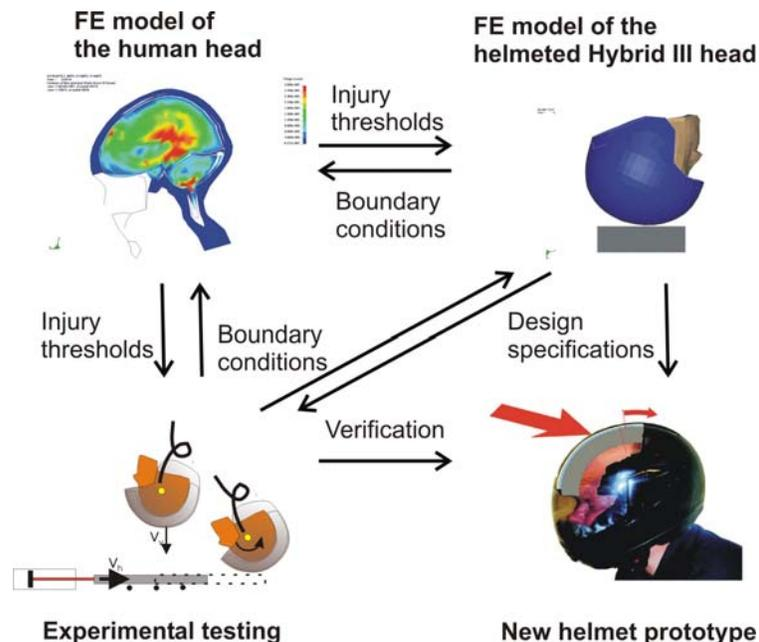
**Figure 4** Design scheme used to improve a safety helmet for oblique impacts.
