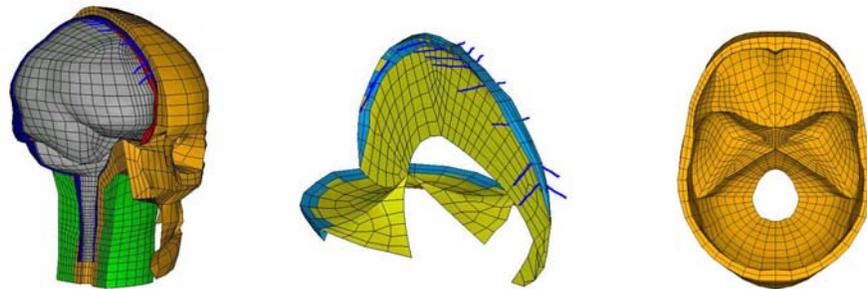
**Figure 5:** Finite element mesh of: a) The human head; b) falx and tentorium including transverse and superior sagittal sinuses with bridging veins; c) Skull bone.
