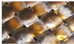
Figure 2: Plain weave CFRP.
