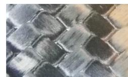
Figure 3: Twill CFRP.
