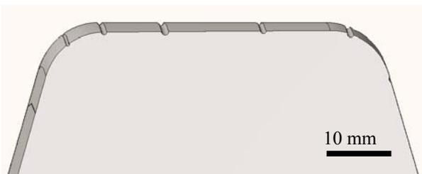
Figure 8. A reconstructed hob for imitating a worn hob. The picture shows the top of the tooth (the protuberance).
