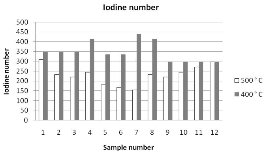
Figure 2: Iodine number of carbons activated using  $H_3PO_4$
