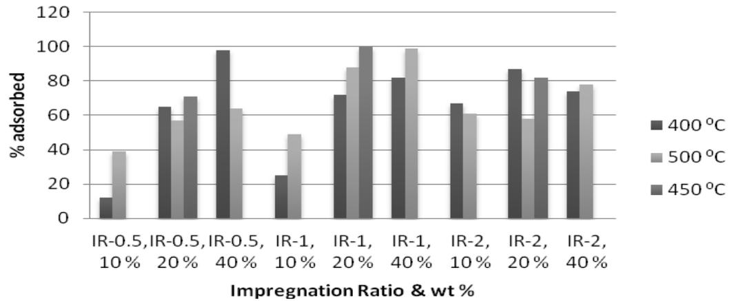
Figure 3: Iodine number of carbons activated using zinc sulphate
