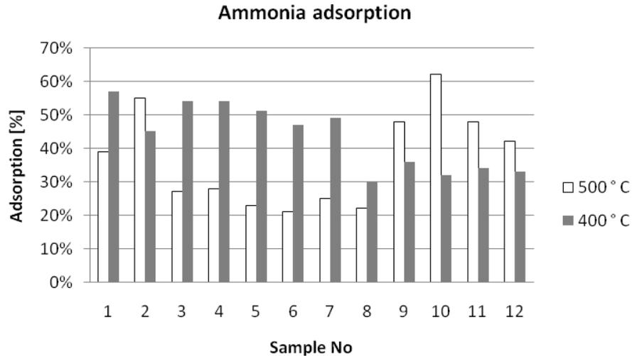
Figure 1: Ammonia adsorption on carbons activated using  $H_3PO_4$
