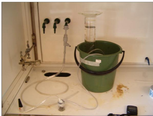
Figure 3 - System of hydrogen production
