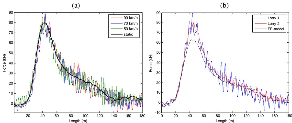
Fig.7 (a) axial force in hanger 1E during passage of lorry1 at different speeds; (b) lorry1 and lorry2 at 90 km/h compared with FE-model simulation result
