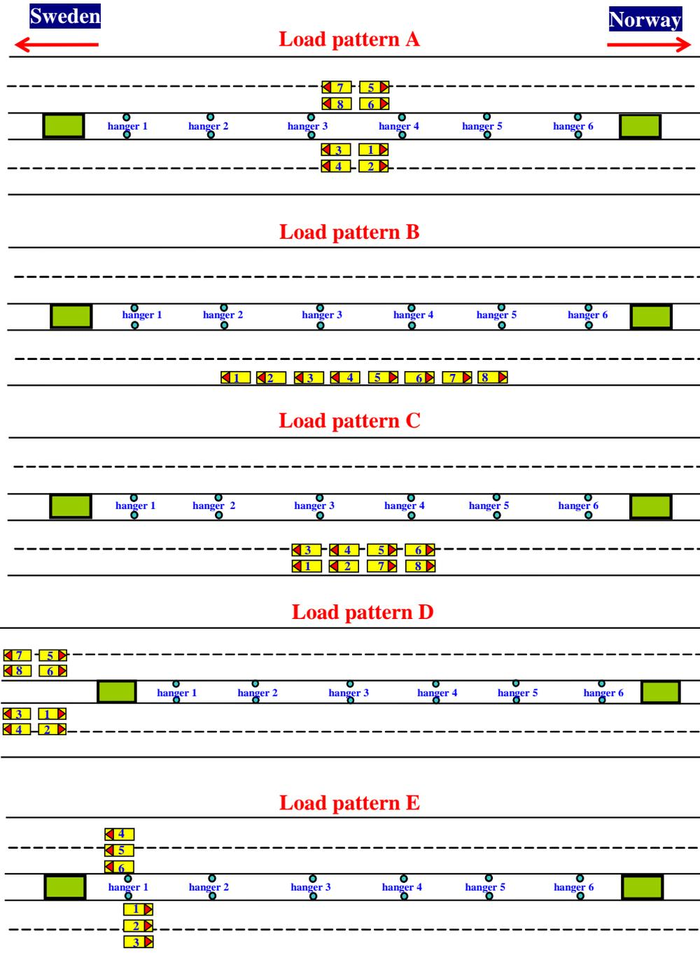
Fig.3 The 5 main loading patterns A-E showing lorry positions on the bridge. As can be seen, the lorries were positioned back-to-back in order to have a symmetric loading and for maximum load effects.
