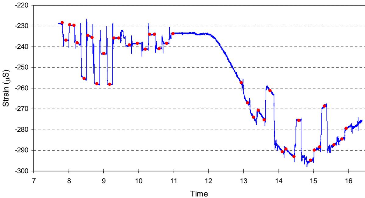
Fig.6 Strain at top of arch segment S6 which is just below the bridge deck on the Swedish side. The red dots indicate the different loaded and unloaded readings made according to Table 1.
