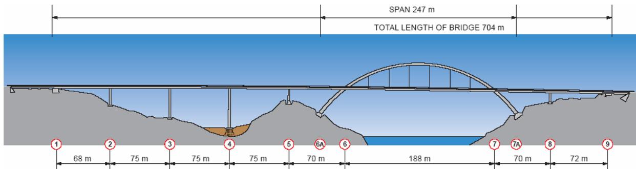
Fig.1 Sketch of the New Svinesund Bridge in its entirety, showing gridline numbering and dimensions.
