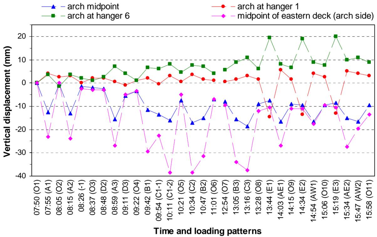
Fig.5 Arch and bridge deck vertical displacements. Hanger 1 corresponds to arch 1/4-point on Swedish side and hanger 6 to arch 1/4-point on Norwegian side.
