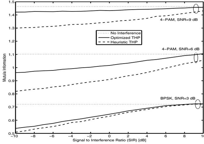
Fig. 6. Mutual information of the optimized THP versus heuristic THP for binary ( $M = 2$ ) and quaternary ( $M = 4$ ) signaling with Gaussian interference and Gaussian noise.
