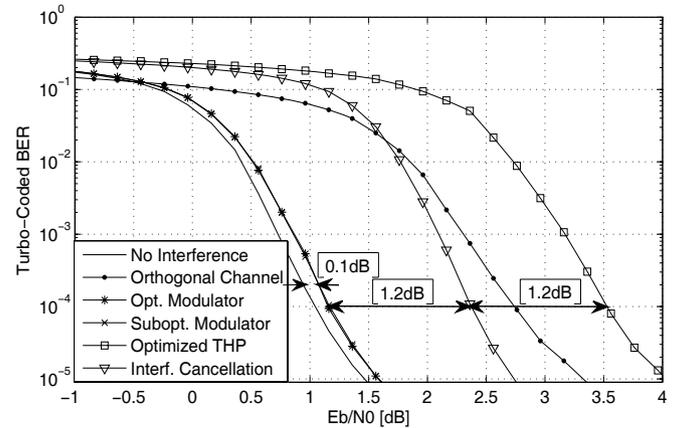
Fig. 4. BER of binary signaling in binary interference with a rate-1/3 turbo code with  $\text{INR}(P_z/\sigma^2) = 6$  dB.
