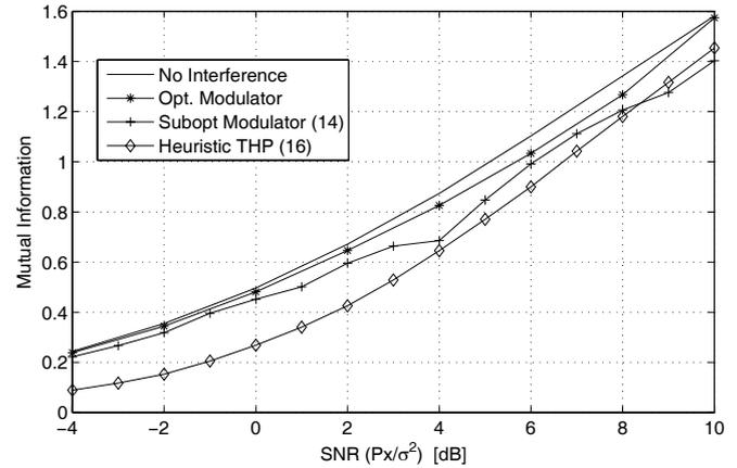
Fig. 3. Mutual information for quaternary signaling in binary interference, with  $\text{INR}(P_z/\sigma^2) = 6$  dB.
