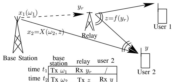
Fig. 1. The base station transmits  $\omega_1$  to user 1 during time slot  $t_1$  and  $\omega_2$  to user 2 during time slot  $t_2$ . The relaying signal  $z=f(y_r)$  dedicated for user 1 appears as “interference” for user 2. With non-causal knowledge of  $z$ , the base station can design a DPC modulator  $x_2 = X(\omega_2, z)$  given the information symbol  $\omega_2$  and the interference  $z$ .
