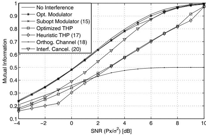
Fig. 2. Mutual information for binary signaling in binary interference, with  $\text{INR}(P_z/\sigma^2) = 6$  dB.
