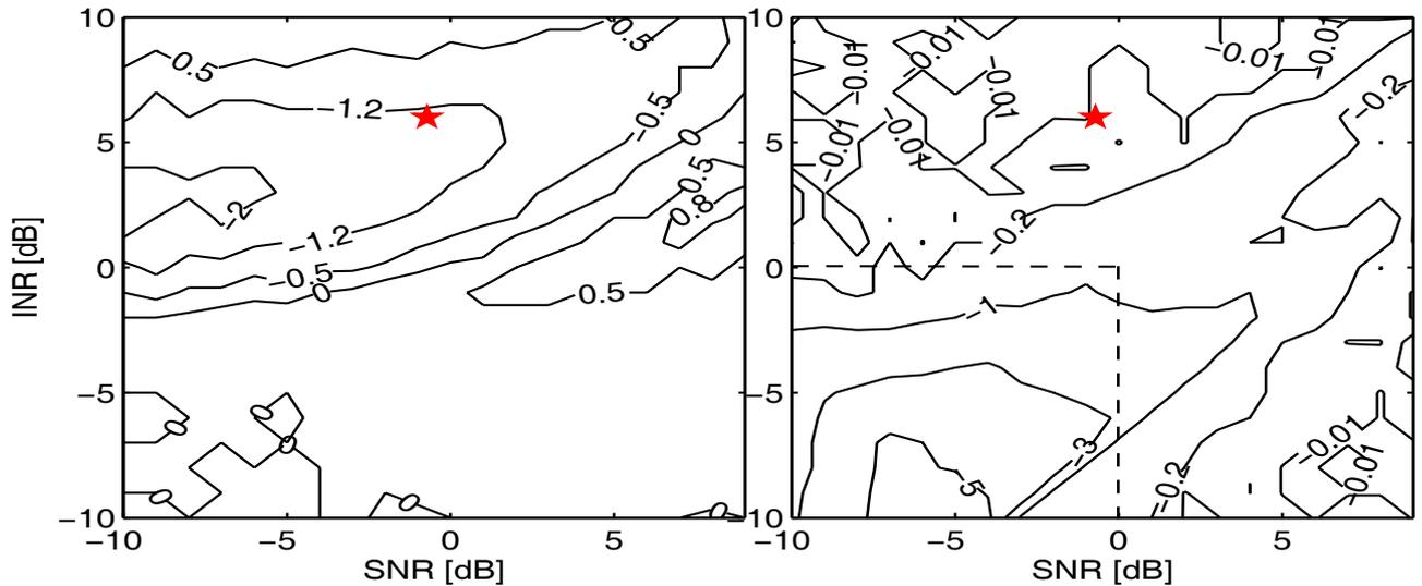
Fig. 5. Energy efficiency (difference in terms of equivalent SNR, in dB) of interference-cancellation (left) and the sub-optimal modulator (right) compared to the optimal modulator. A positive number indicates better energy efficiency.
