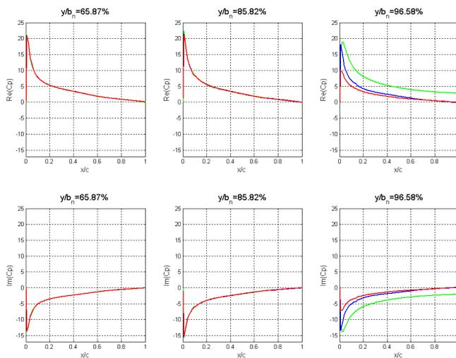
Figure 14: Real and Imaginary part of the pressure coefficient at different location for  $k = 0.01$  (delta value between the upper and the lower wing)
