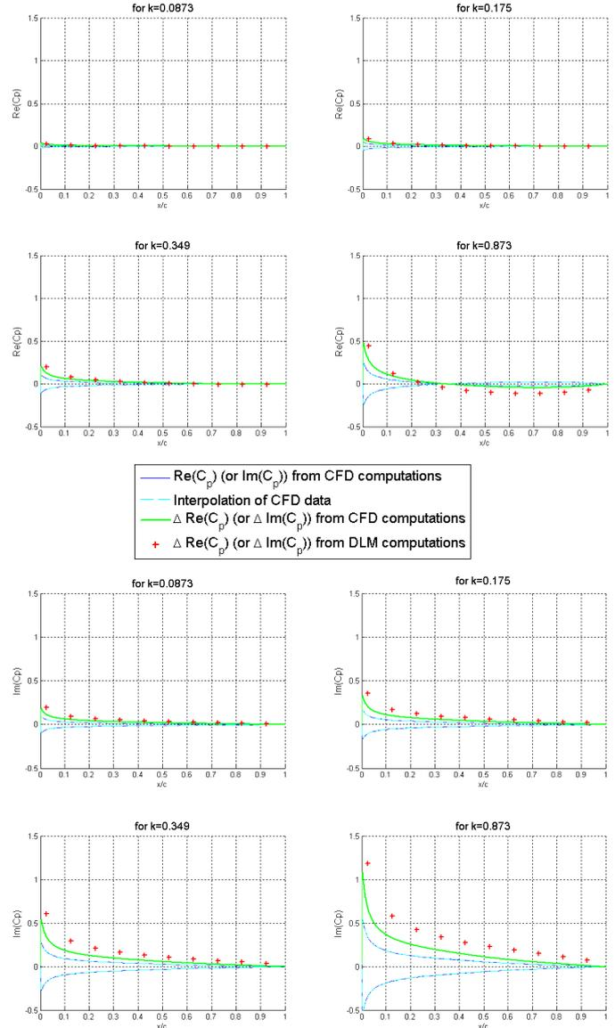
Figure 10: Comparison between CFD and DLM in forced motion ( $Ma = 0.5$ )
