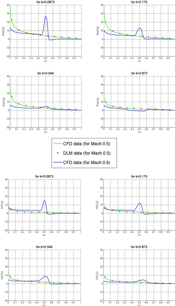
Figure 9: Comparison between two different mach numbers for CFD computations
