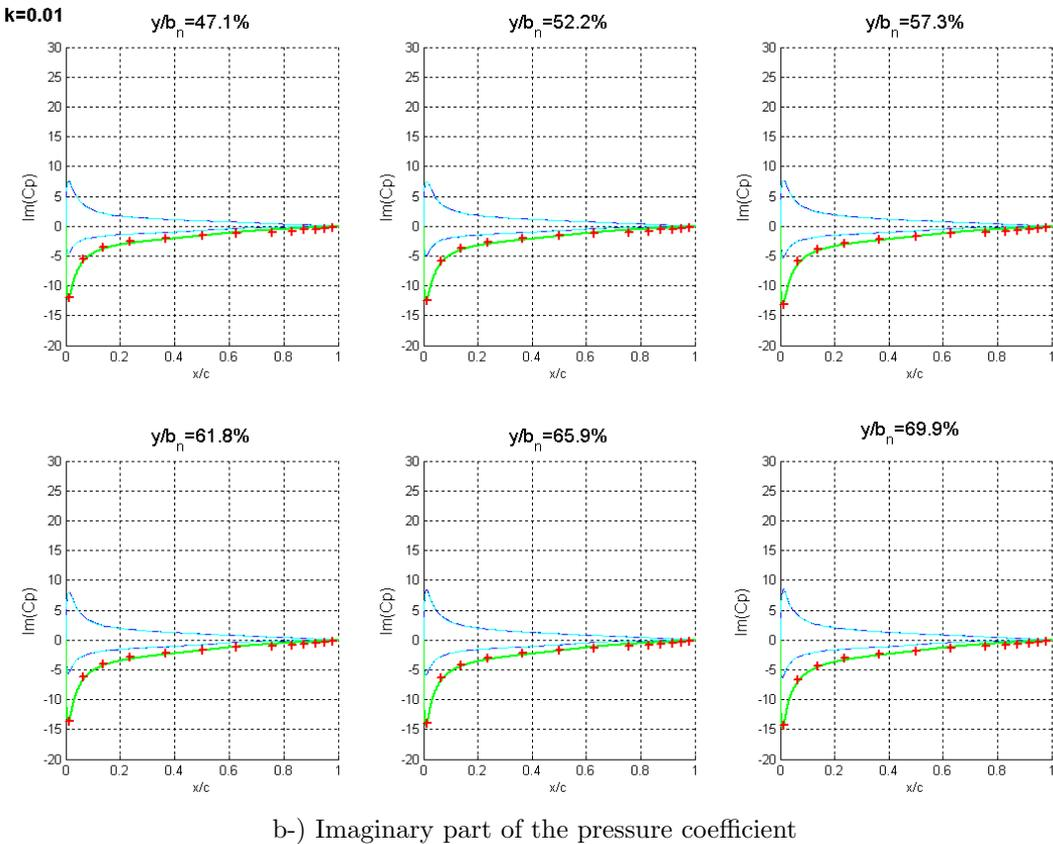
Figure 27: Comparison between CFD and DLM data for a reduced frequency  $k = 0.010$
