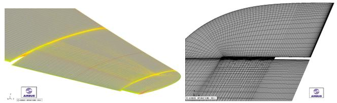
Figure 6: Movable aileron with hole and details at the wing tip
