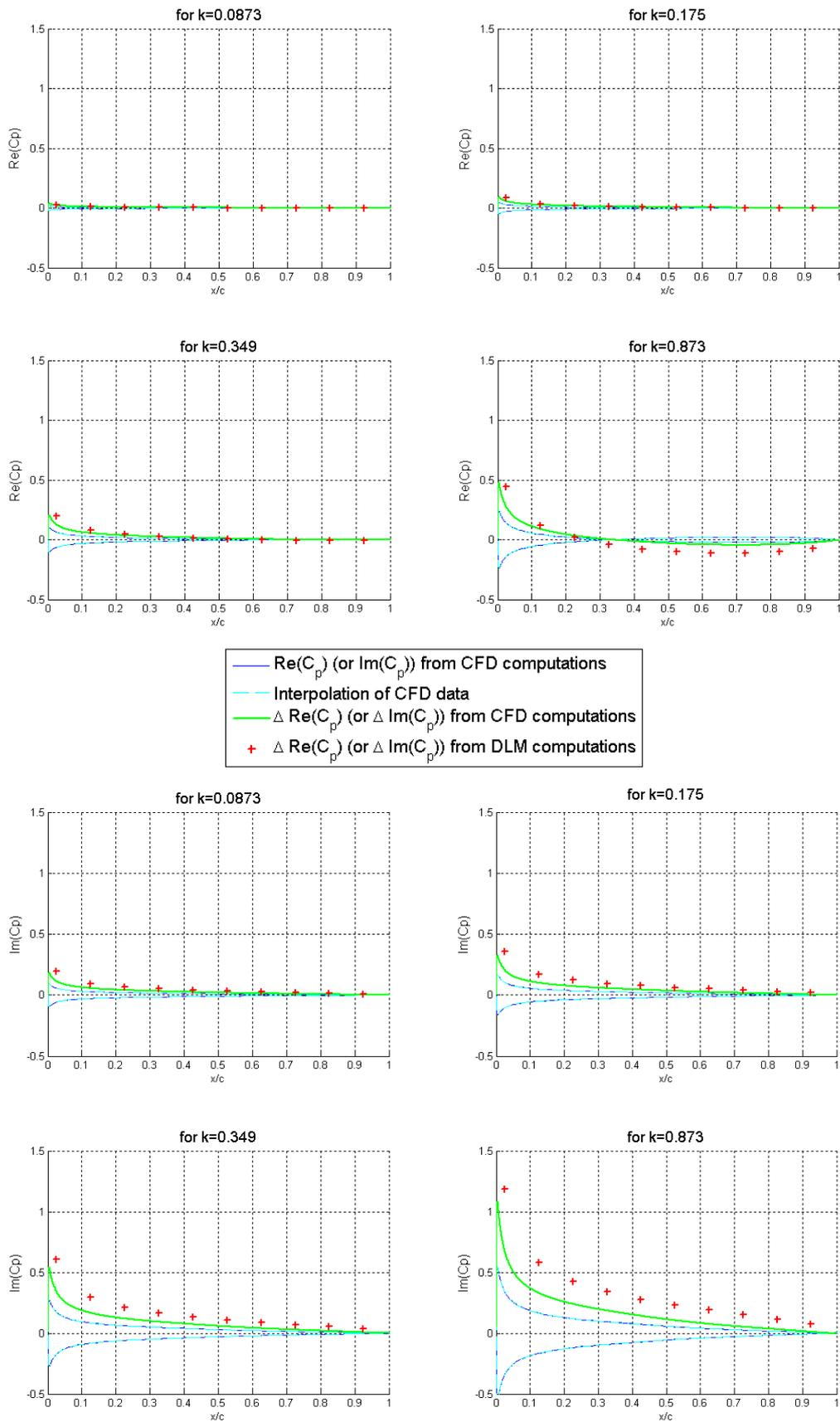
Figure 26: Comparison between CFD and DLM in forced motion ( $Ma = 0.5$ )
