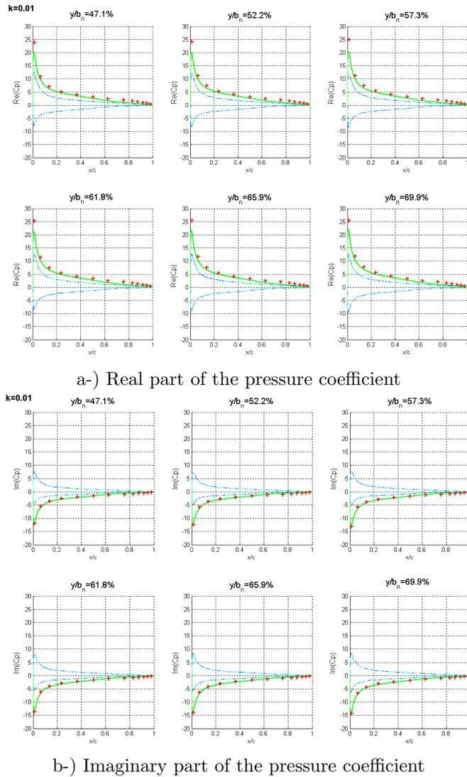
Figure 11: Comparison between CFD and DLM data for a reduced frequency  $k = 0.010$
