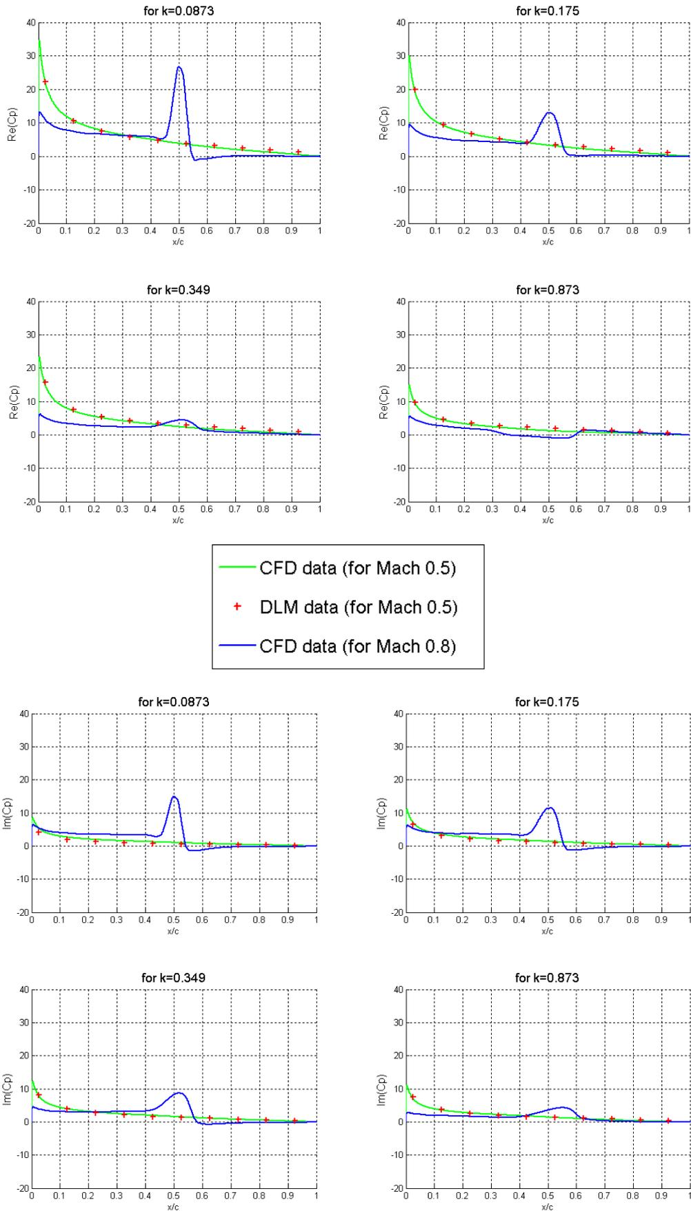
Figure 25: Comparison between two different mach numbers for CFD computations
