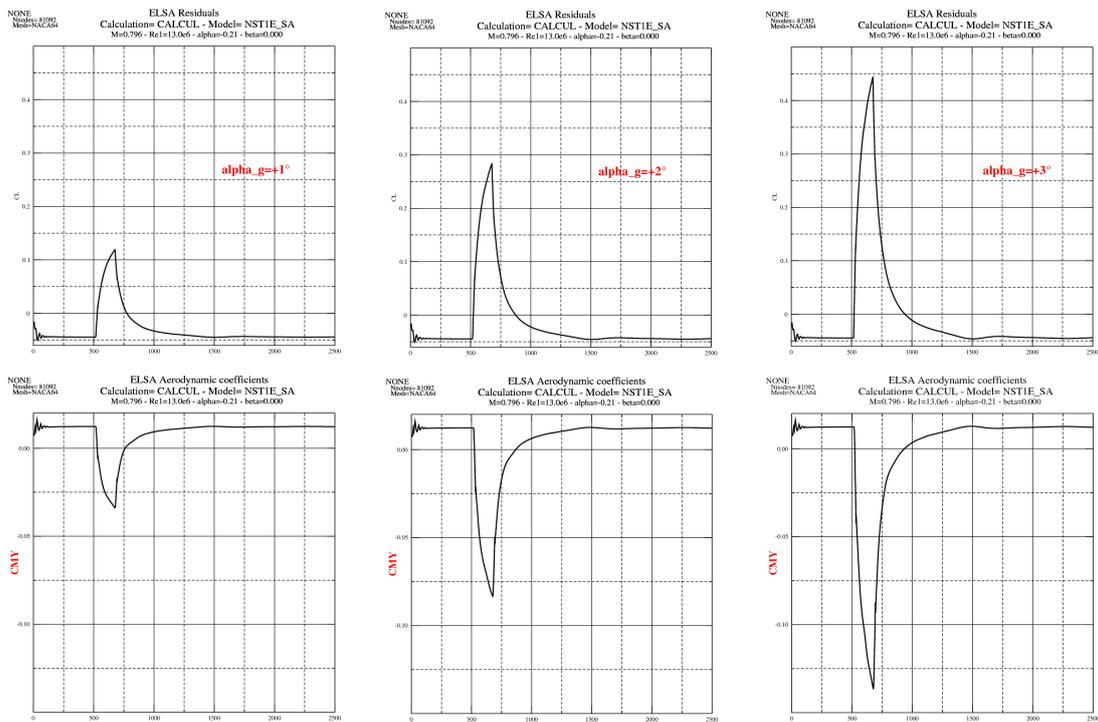
Figure 19: Lift and moment coefficients, "sharp - edged" gust response (impact of wavelength)
