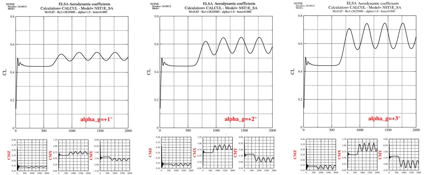
Figure 22: Lift and moment coefficients, harmonic gust response (impact of wavelength)
