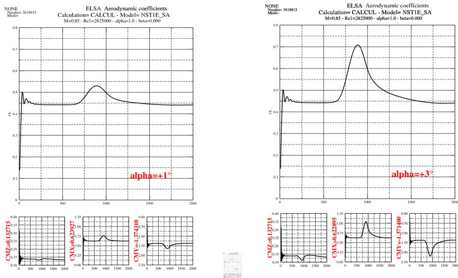
Figure 21: Lift and moment coefficients, "1 - cos" discrete gust response (impact of wavelength)
