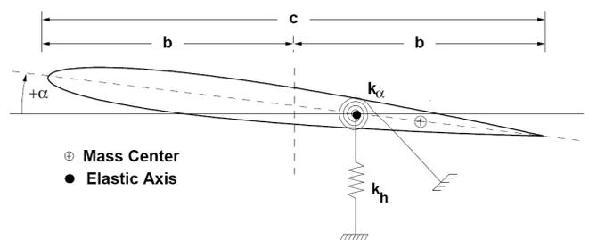
Figure 4: Geometry for typical two-Degree-of-Freedom (2-DOFs) airfoil profile model (from [4])
