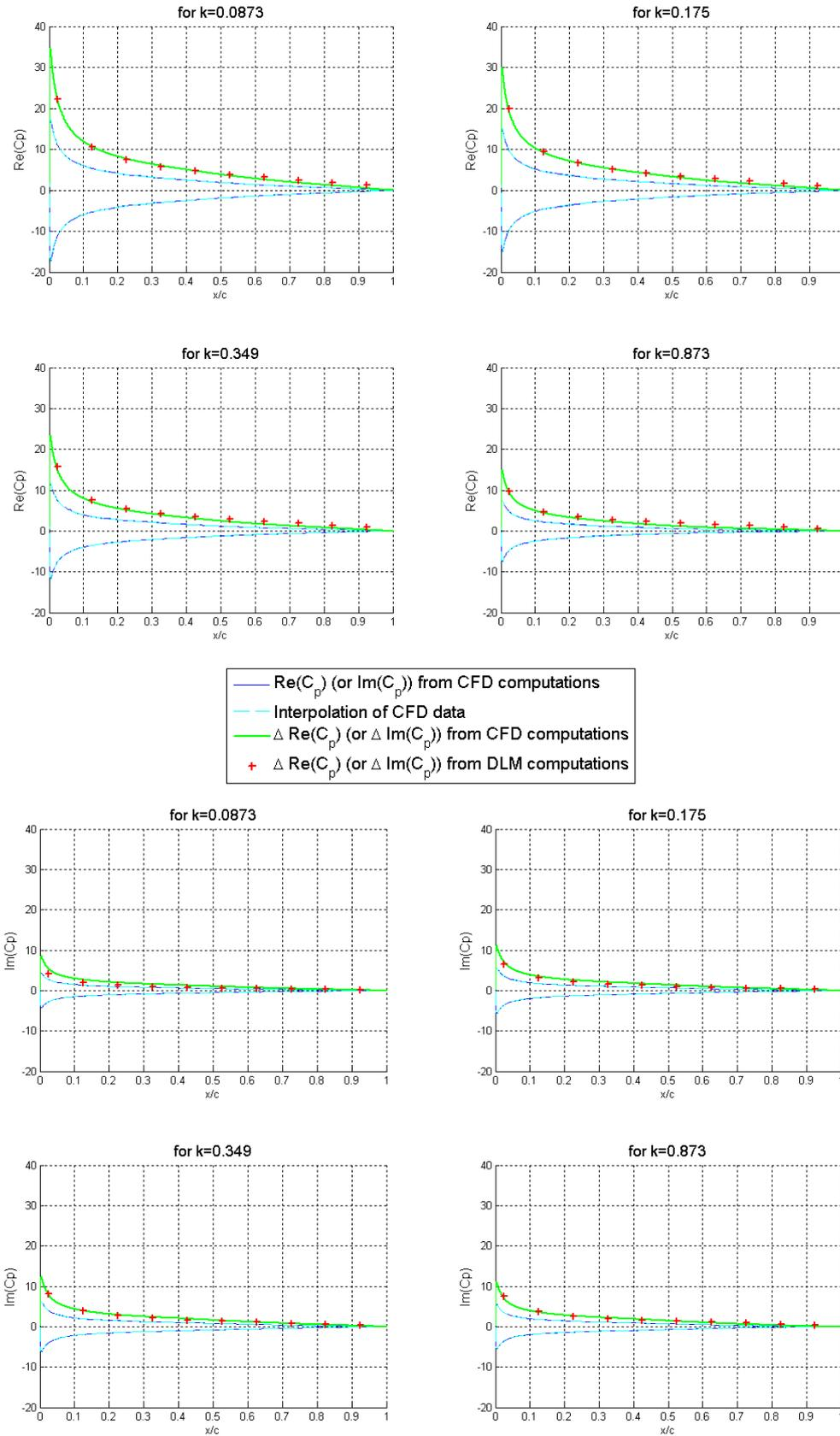
Figure 24: Comparison between CFD and DLM data for  $Ma = 0.5$  (gust response)
