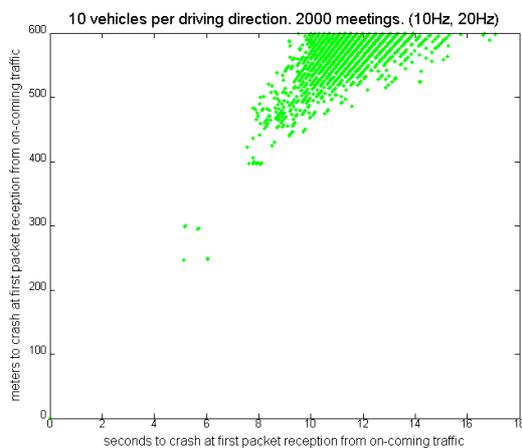
Figure 8: Simulation results when having 10 Hz send rate of leading vehicles and 20 Hz of non-leading vehicles.
