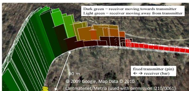
Figure 4: Measurement results for stationary transmitter and mobile receiver. Achieved transmission range at limited LOS around a vegetated curve. (Google Earth visualization).
