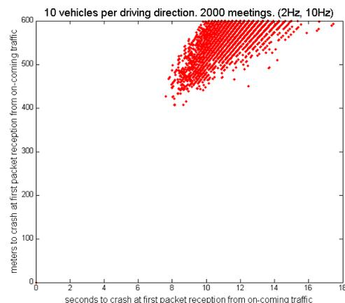
Figure 6: Simulation results when having 2 Hz send rate of leading vehicles and 10 Hz of non-leading vehicles.
