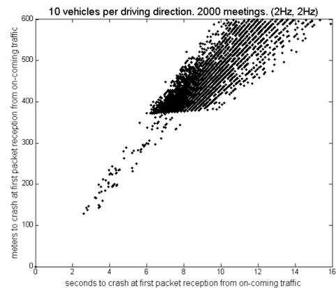
Figure 5: Simulation results when having 2 Hz send rate of both leading vehicles and non-leading vehicles.
