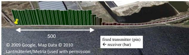
Figure 3: Measurement results for stationary transmitter and mobile receiver. Achieved transmission range at full LOS. (Google Earth visualization).
