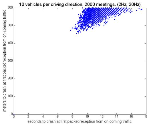
Figure 7: Simulation results when having 2 Hz send rate of leading vehicles and 20 Hz of non-leading vehicles.
