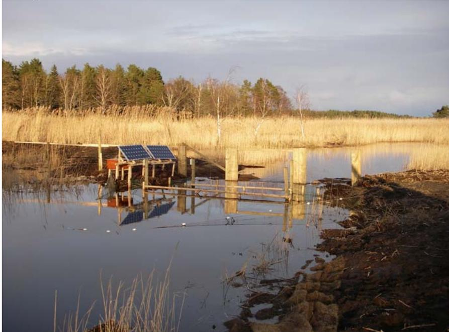
FIG. 9 PIT-TAG station powered by solar panels, recording returning pike after a year in the Baltic Sea (Photo: Olof Engstedt)
