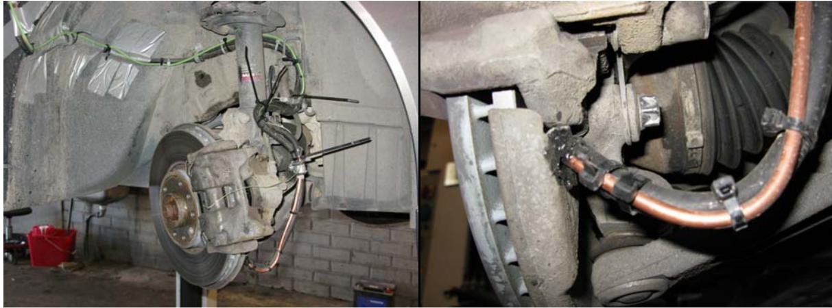
*Figure 2. Photo of the test tubes for particle measurements mounted directly after the piston side brake pad on the piston side.*
