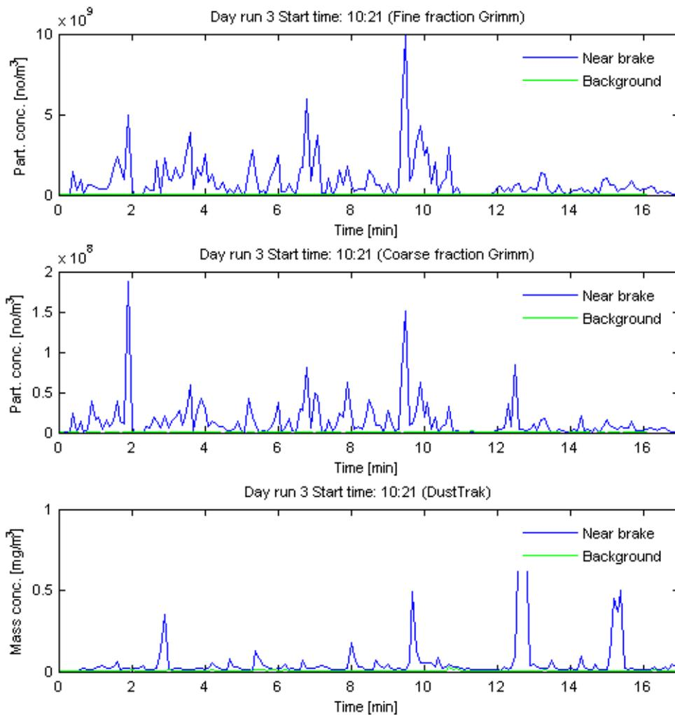
Figure 25. Fine and coarse fraction particle concentrations as measured by the GRIMM instrument during the test time and the mass concentration as measured by the DustTrak instrument. The blue graphs are the concentrations measured near the brake and the green graphs are the measured background concentration.
