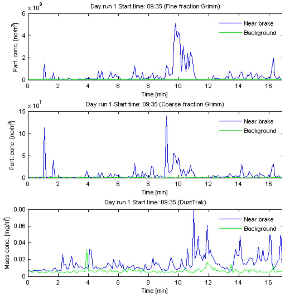
Figure 17. Fine and coarse fraction particle concentrations as measured by the GRIMM instrument during the test time and the mass concentration as measured by the DustTrak instrument. The blue graphs are the concentrations measured near the brake and the green graphs are the measured background concentration.
