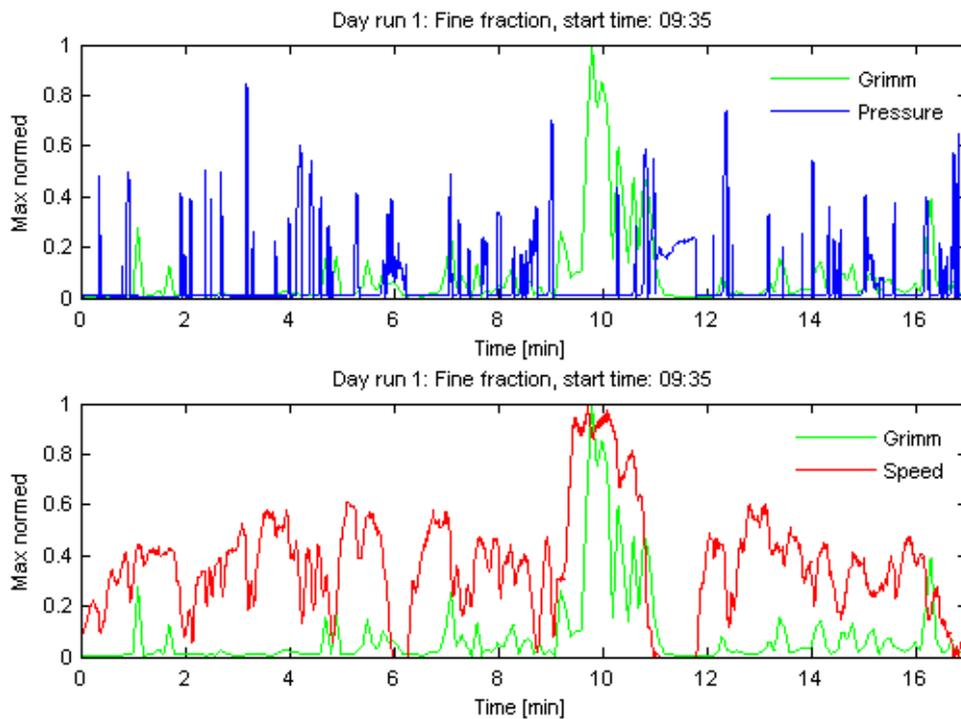
Figure 15. The green graph is the fine fraction particle concentrations as measured by the GRIMM instrument, the blue graph is the measured brake cylinder pressure, and the red graph is the measured speed of the car.
