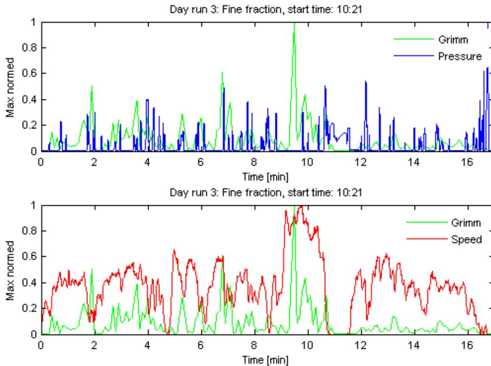
Figure 23. The green graph is the fine fraction particle concentrations as measured by the GRIMM instrument, the blue graph is the measured brake cylinder pressure, and the red graph is the measured speed of the car.
