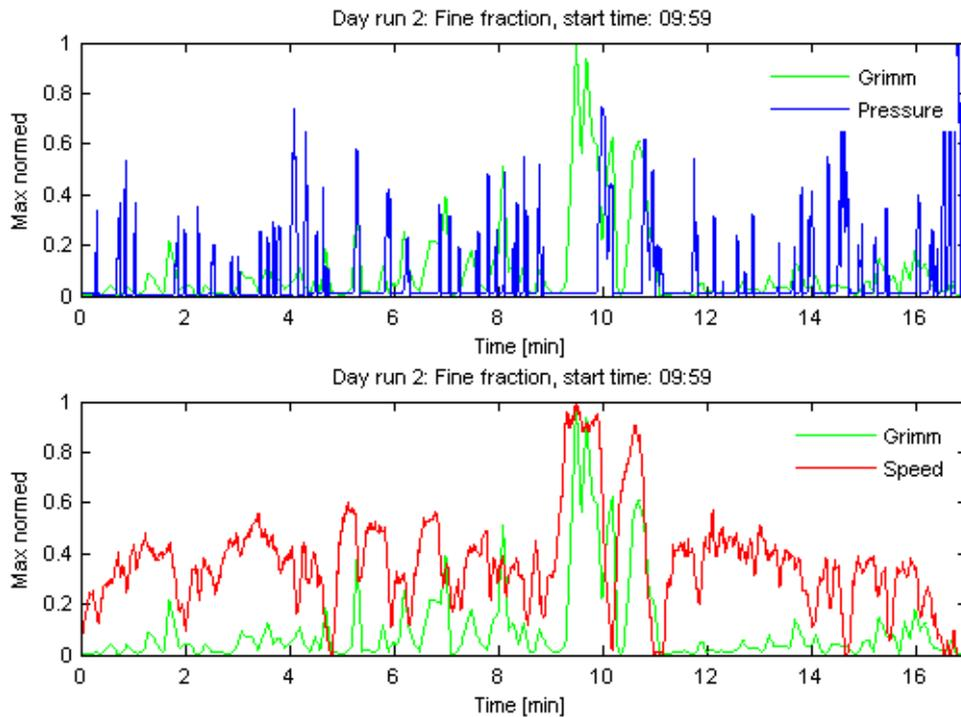
Figure 19. The green graph is the fine fraction particle concentrations as measured by the GRIMM instrument, the blue graph is the measured brake cylinder pressure, and the red graph is the measured speed of the car.
