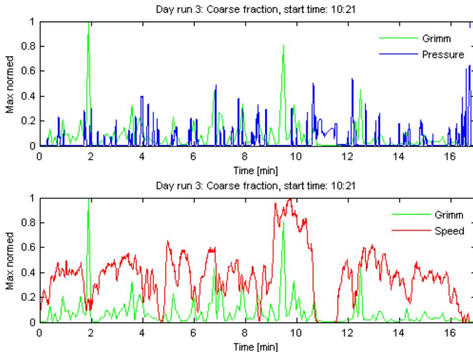
Figure 24. The green graph is the coarse fraction particle concentrations as measured by the GRIMM instrument, the blue graph is the measured brake cylinder pressure, and the red graph is the measured speed of the car.
