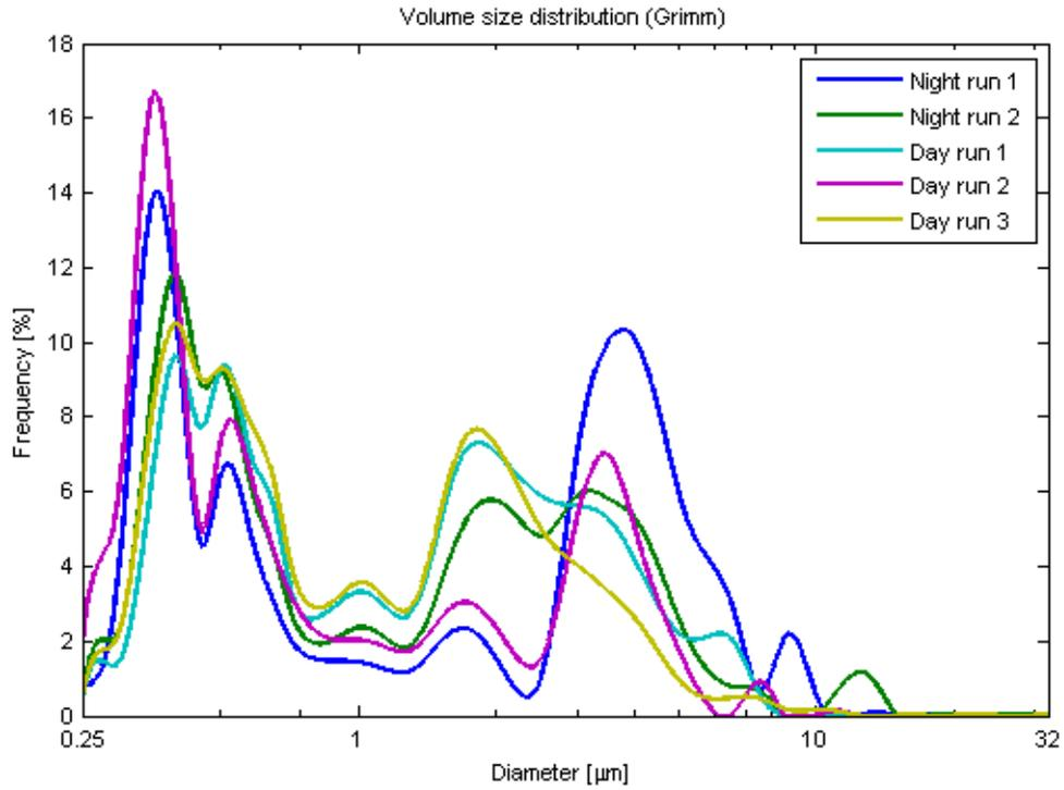
Figure 6. Mean normalized volume size distributions as measured with the GRIMM instrument.
