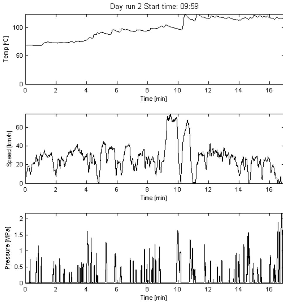
Figure 22. Finger side pad temperature, car speed and brake cylinder pressure measured during the test run.
