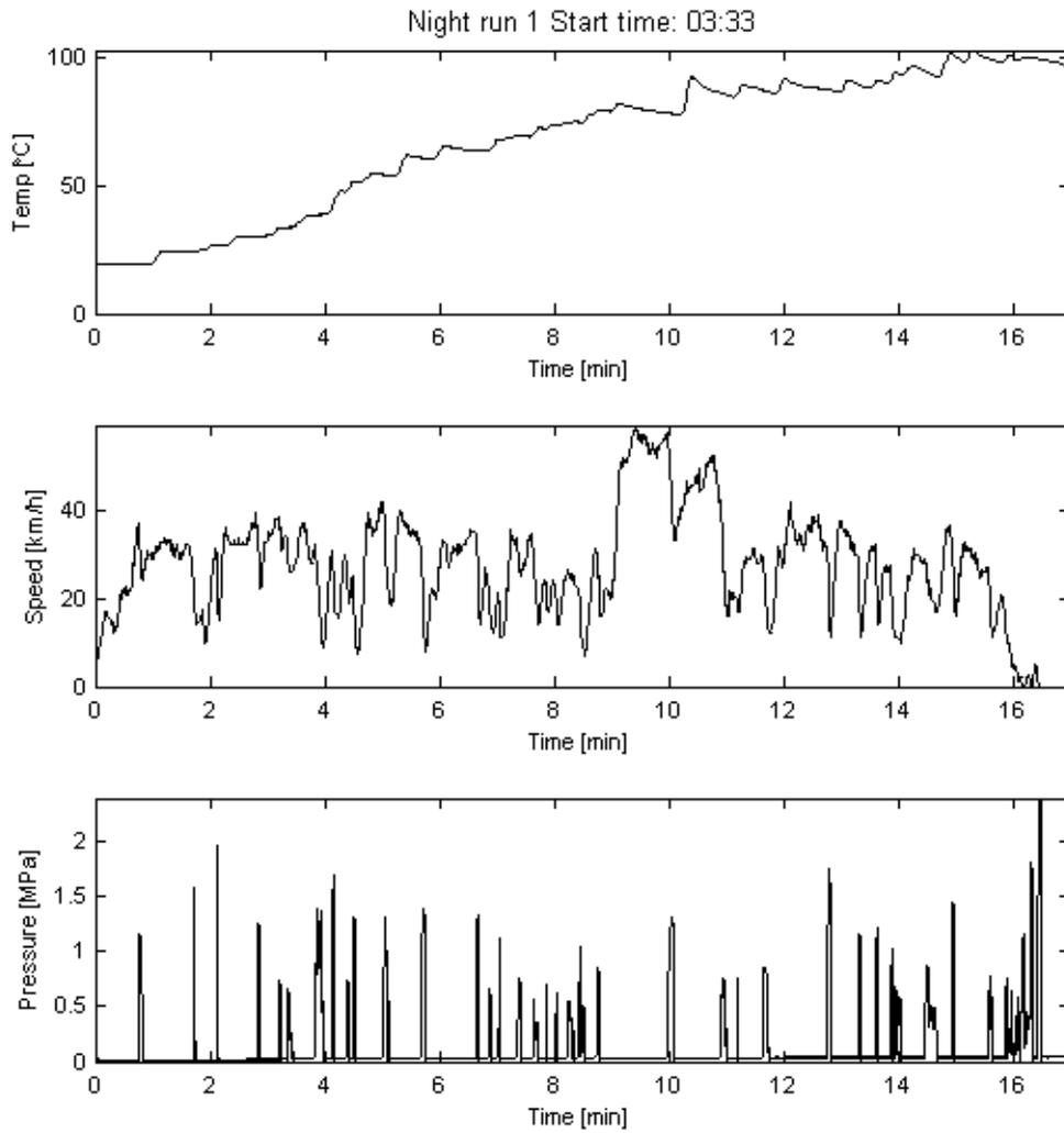
Figure 10. Finger side pad temperature, car speed and brake cylinder pressure measured during the test run.
