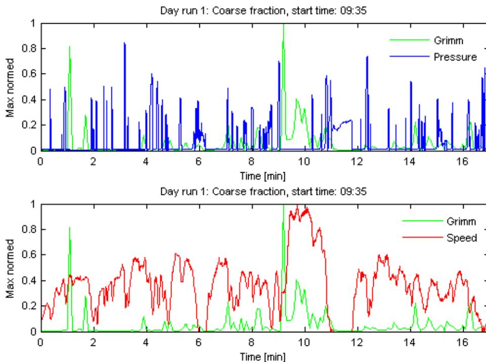
Figure 16. The green graph is the coarse fraction particle concentrations as measured by the GRIMM instrument, the blue graph is the measured brake cylinder pressure, and the red graph is the measured speed of the car.
