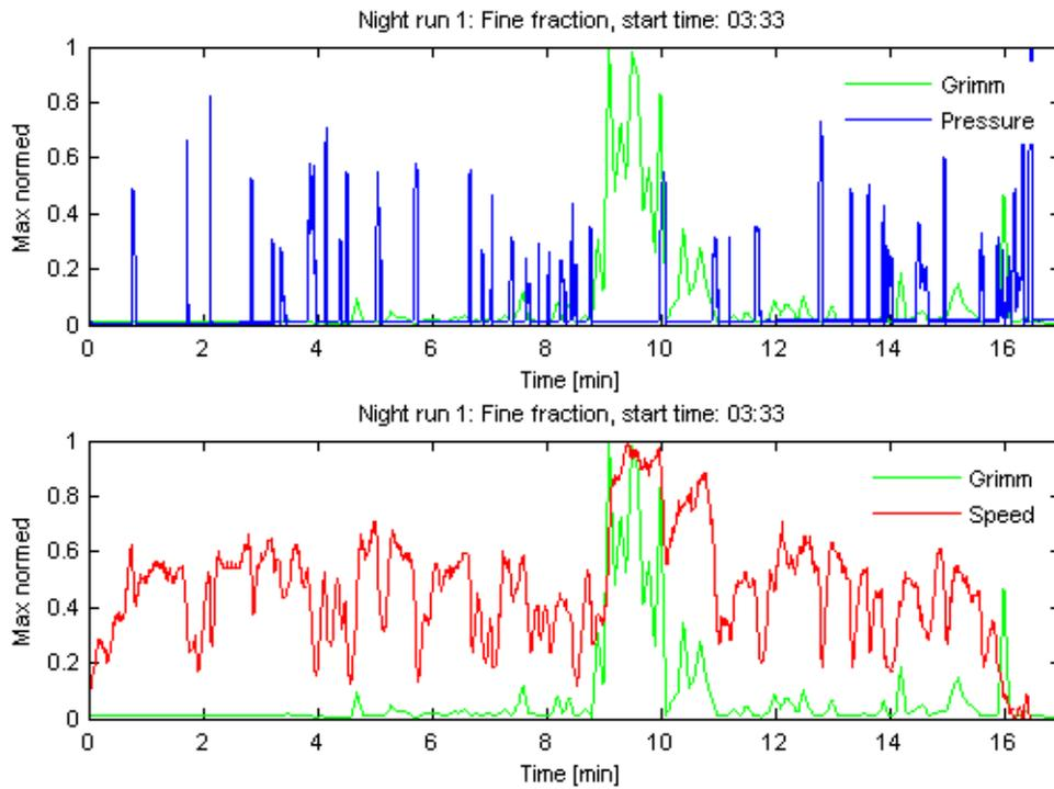
Figure 7. The green graph is the fine fraction particle concentrations as measured by the GRIMM instrument, the blue graph is the measured brake cylinder pressure, and the red graph is the measured speed of the car.
