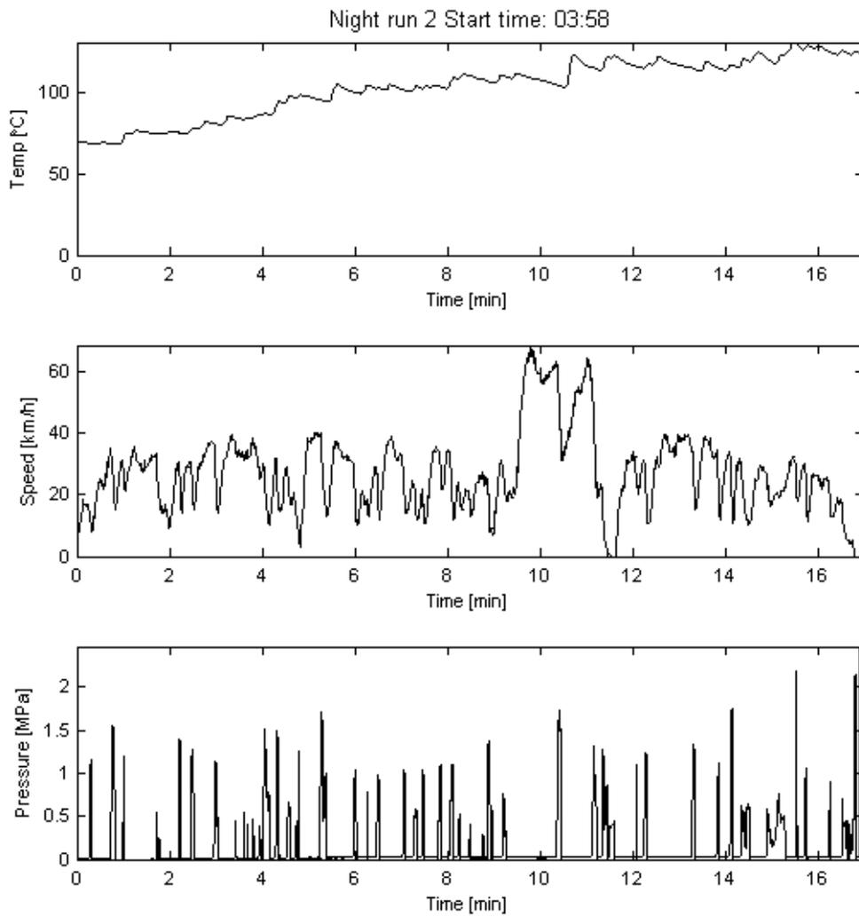
Figure 14. Finger side pad temperature, car speed and brake cylinder pressure measured during the test run.
