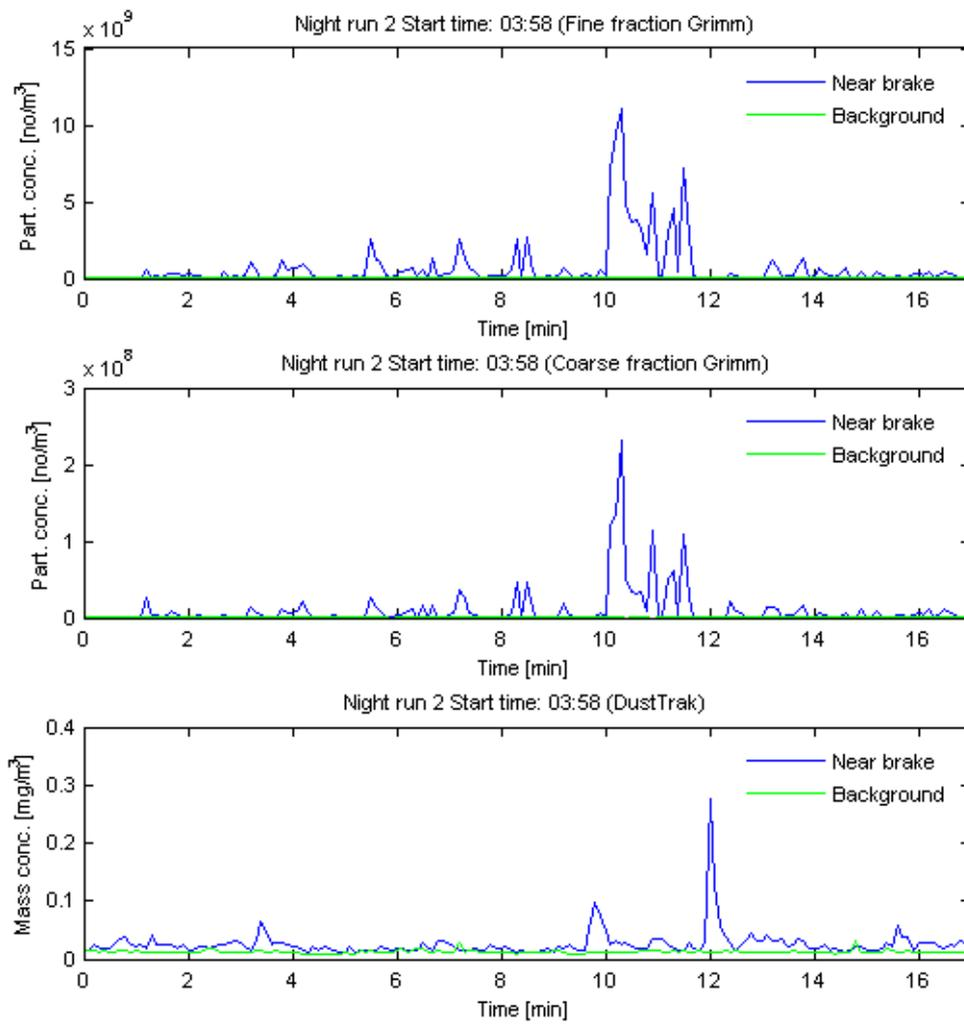
Figure 13. Fine and coarse fraction particle concentrations as measured by the GRIMM instrument during the test time and the mass concentration as measured by the DustTrak instrument. The blue graphs are the concentrations measured near the brake and the green graphs are the measured background concentration.
