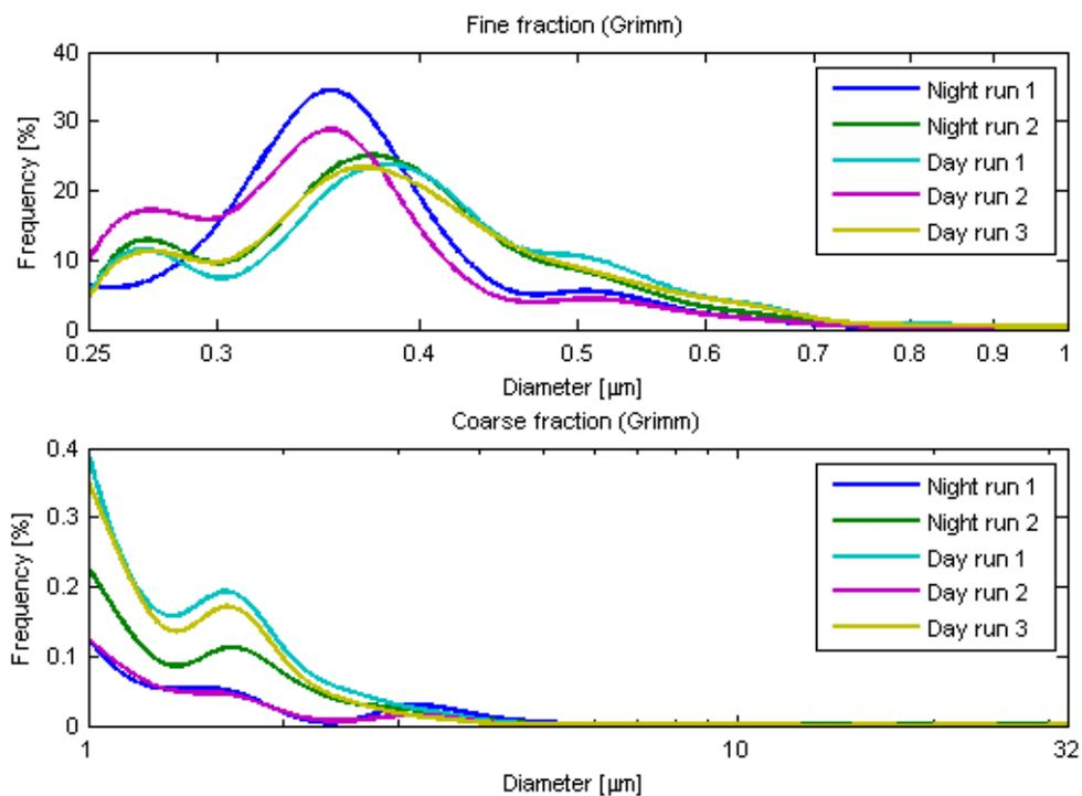
Figure 5. Mean normalized particle size distributions as measured with the GRIMM instrument.
