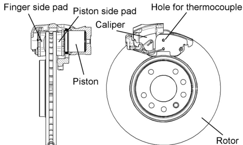
*Figure 1. Disc brake assembly with a single piston floating caliper and a ventilated rotor.*
