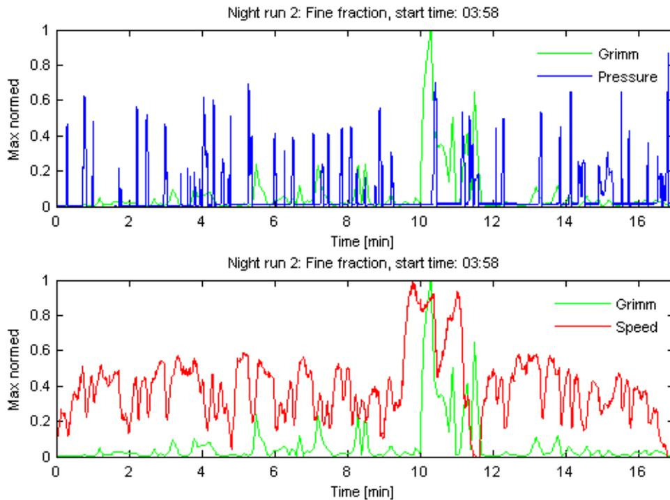
Figure 11. The green graph is the fine fraction particle concentrations as measured by the GRIMM instrument, the blue graph is the measured brake cylinder pressure, and the red graph is the measured speed of the car.
