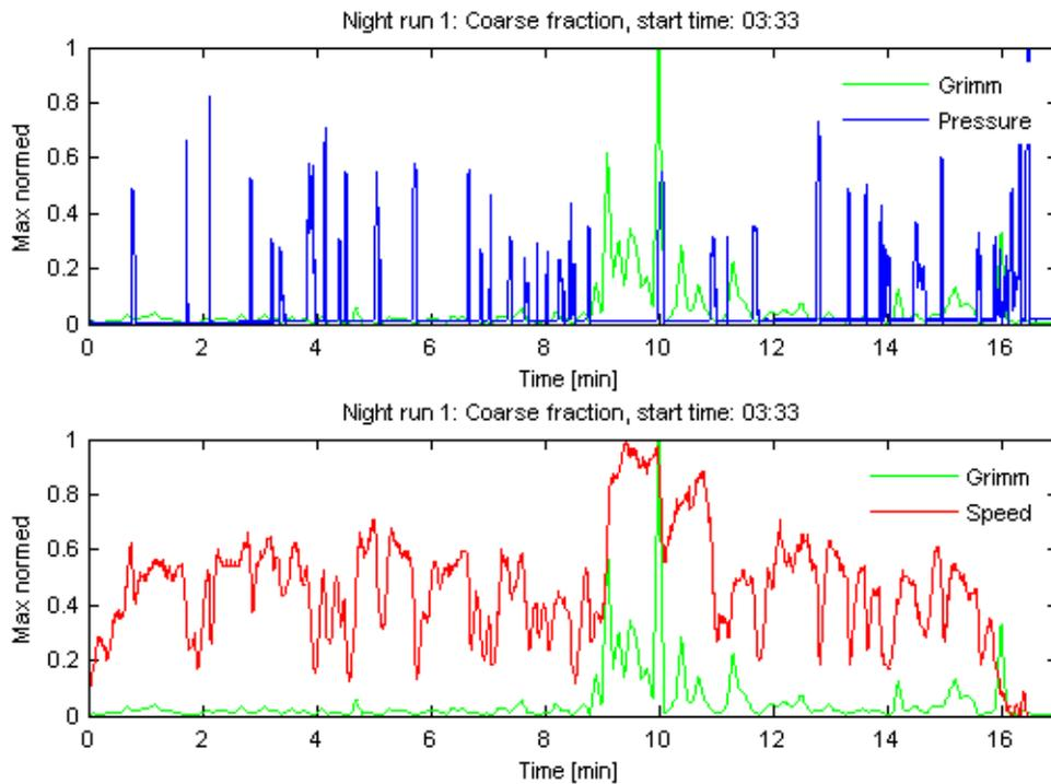
Figure 8. The green graph is the coarse fraction particle concentrations as measured by the GRIMM instrument, the blue graph is the measured brake cylinder pressure, and the red graph is the measured speed of the car.
