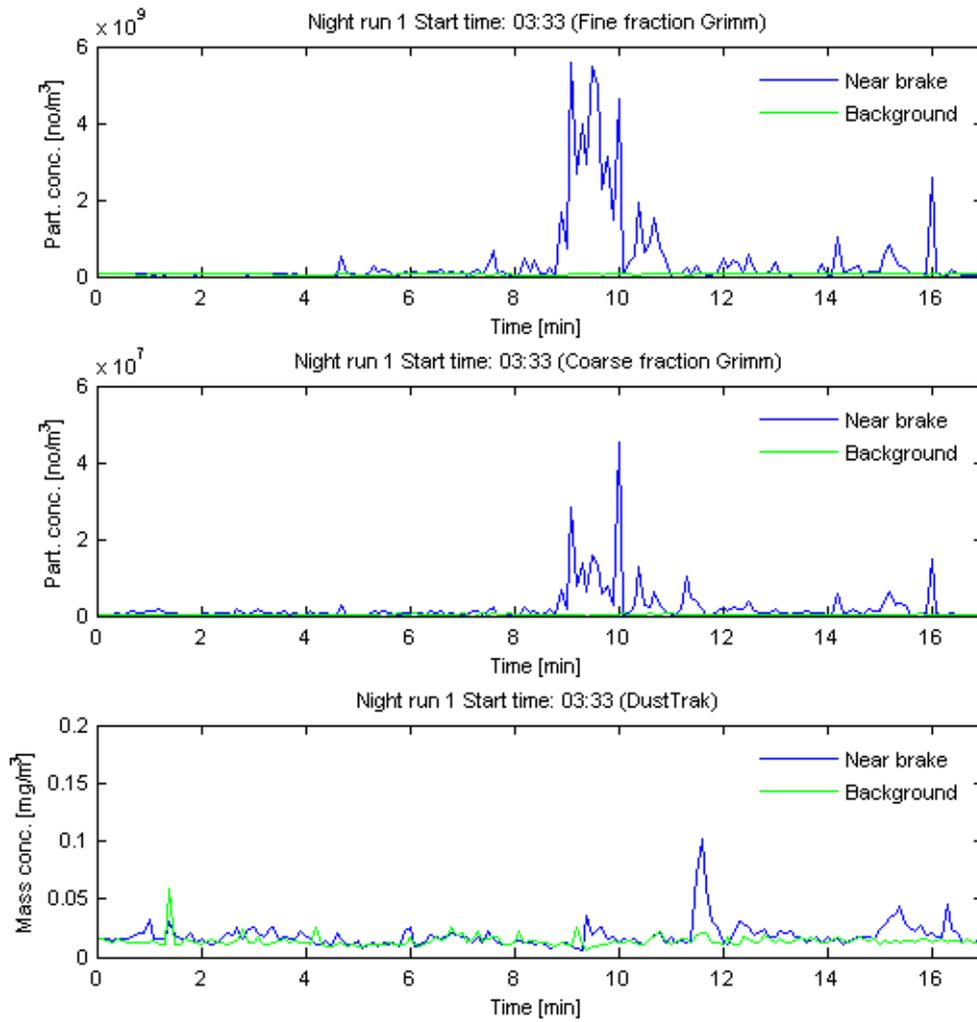
Figure 9. Fine and coarse fraction particle concentrations as measured by the GRIMM instrument during the test time and the mass concentration as measured by the DustTrak instrument. The blue graphs are the concentrations measured near the brake and the green graphs are the measured background concentration.
