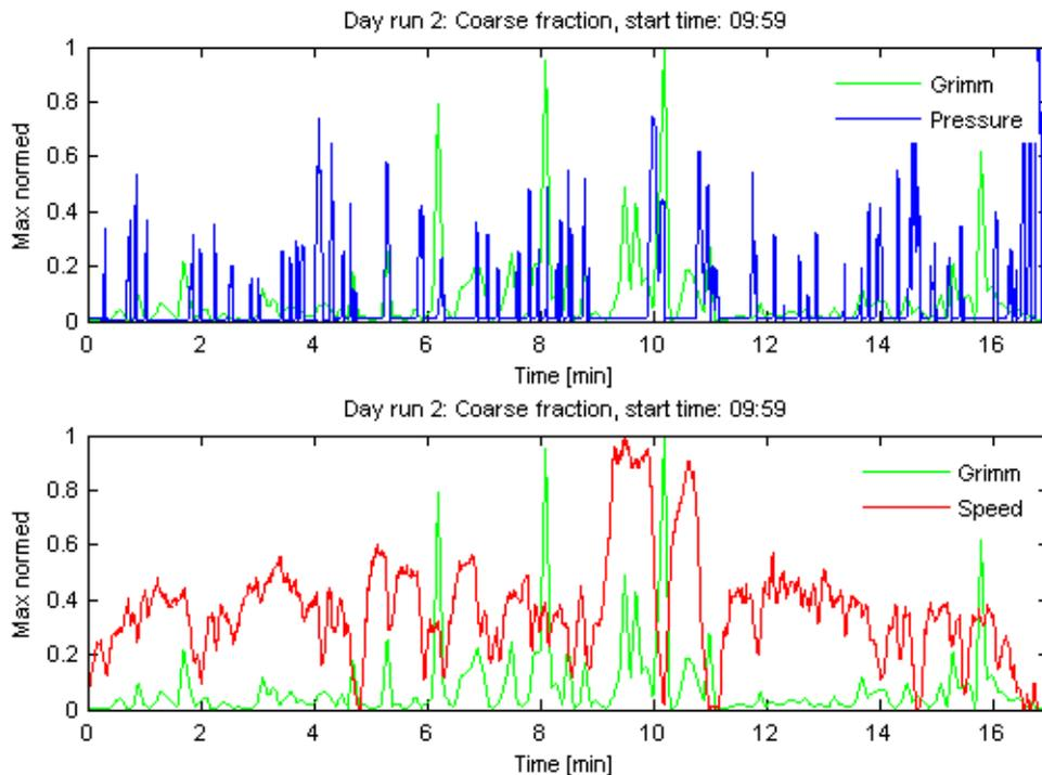
Figure 20. The green graph is the coarse fraction particle concentrations as measured by the GRIMM instrument, the blue graph is the measured brake cylinder pressure, and the red graph is the measured speed of the car.
