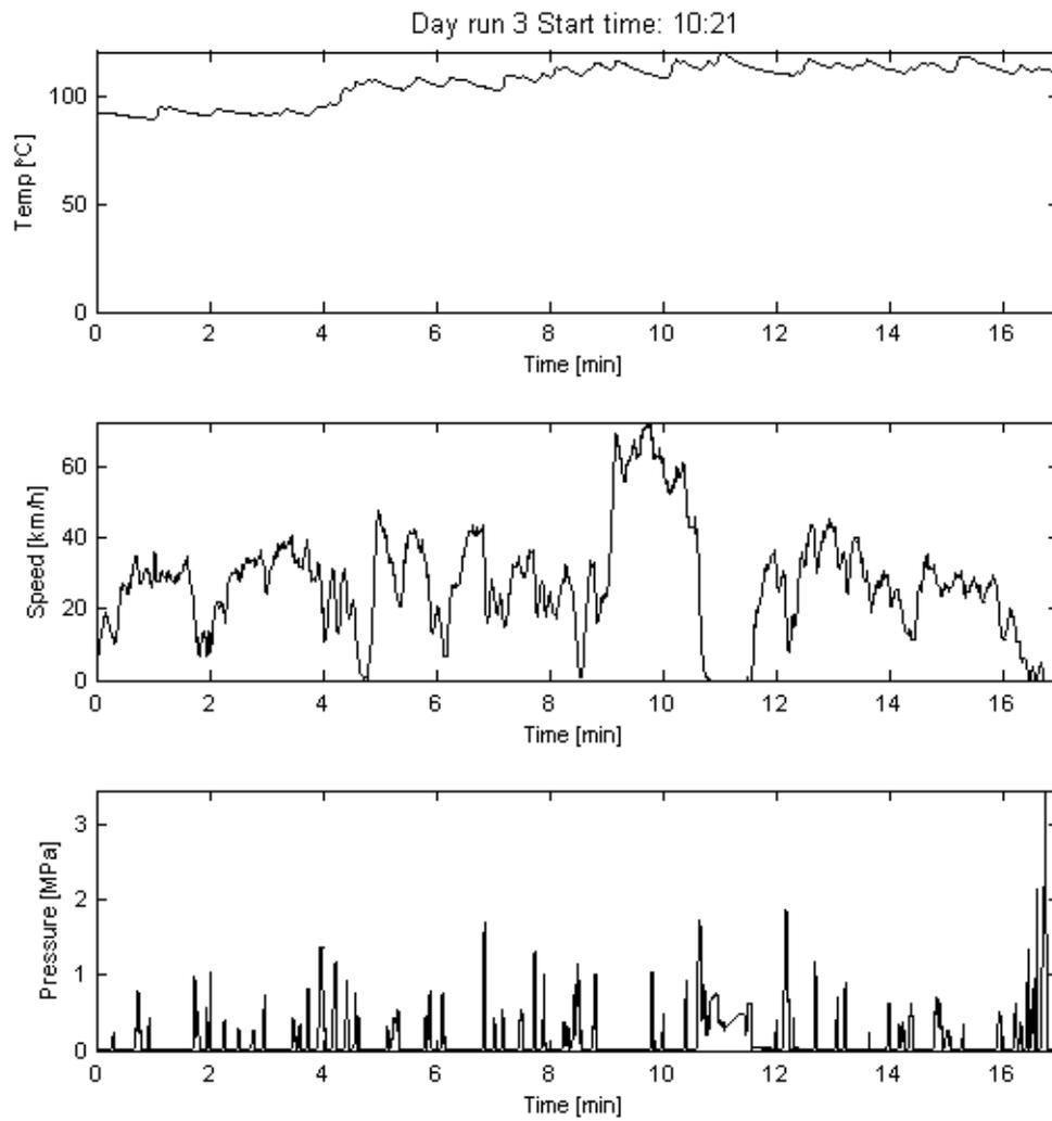
Figure 26. Finger side pad temperature, car speed and brake cylinder pressure measured during the test run.
