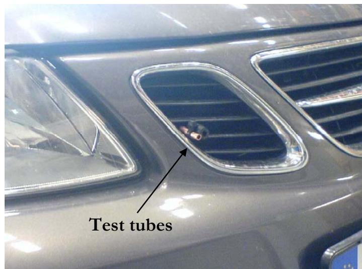
*Figure 3. Photo of the test tubes for measurements of the background particle concentration mounted in the front of the test car.*
