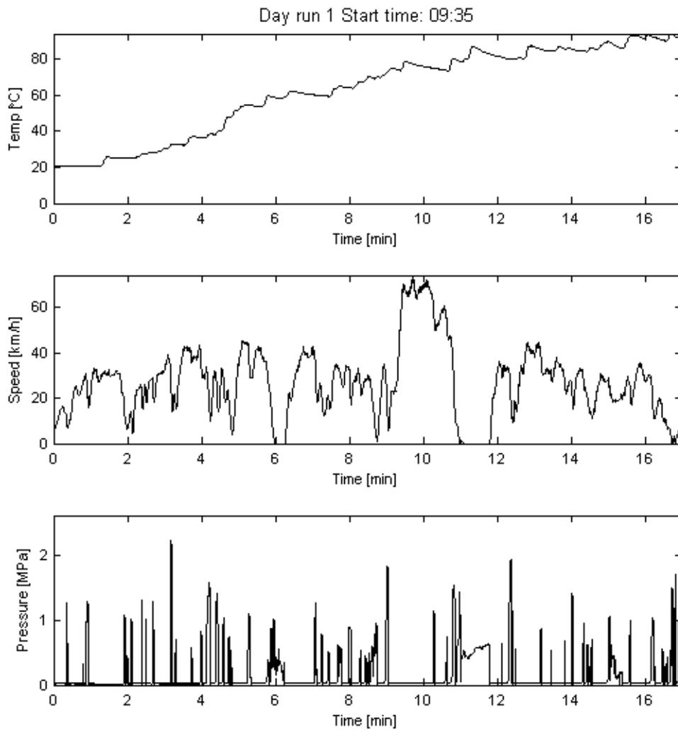
Figure 18. Finger side pad temperature, car speed and brake cylinder pressure measured during the test run.
