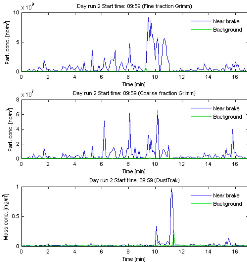
Figure 21. Fine and coarse fraction particle concentrations as measured by the GRIMM instrument during the test time and the mass concentration as measured by the DustTrak instrument. The blue graphs are the concentrations measured near the brake and the green graphs are the measured background concentration.
