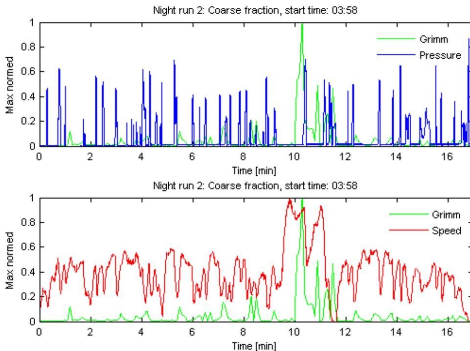
Figure 12. The green graph is the coarse fraction particle concentrations as measured by the GRIMM instrument, the blue graph is the measured brake cylinder pressure, and the red graph is the measured speed of the car.
