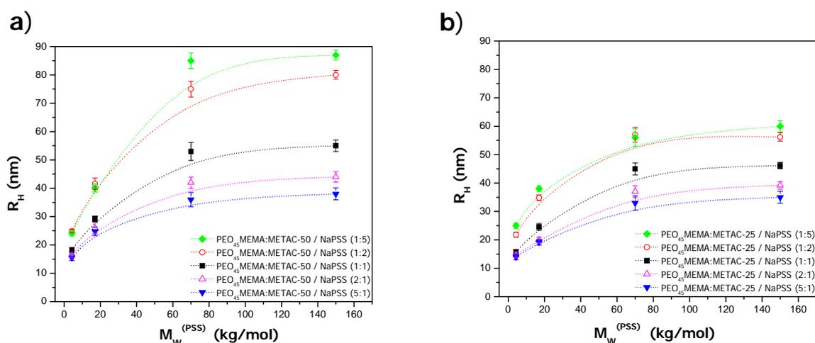
**Figure 4.5** Hydrodynamic radius of complexes containing a) PEO<sub>45</sub>MEMA:METAC-50 and b) PEO<sub>45</sub>MEMA:METAC-25 as a function of PSS molecular mass. The solution contained 5 mM NaCl and 50 ppm of PEO<sub>45</sub>MEMA:METAC-25(50). The dashed curves are plotted as guides for the eye.
