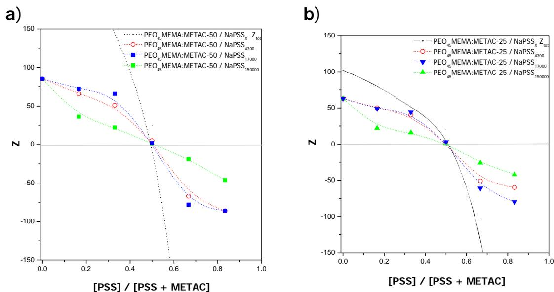
**Figure 4.8** Number of charges ( $Z$ ) and total number of charges ( $Z_{tot}$ ) as a function of PSS content for (a)  $PEO_{45}MEMA:METAC-50/NaPSS_x$  and (b)  $PEO_{45}MEMA:METAC-25/NaPSS_x$  complexes. The concentration of the cationic polymer was fixed to 50 ppm.
