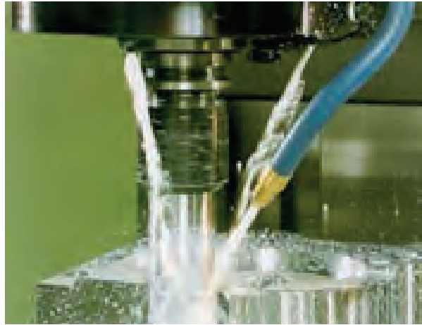
Figure 19: Flood cutting fluids cooling in a milling operation
