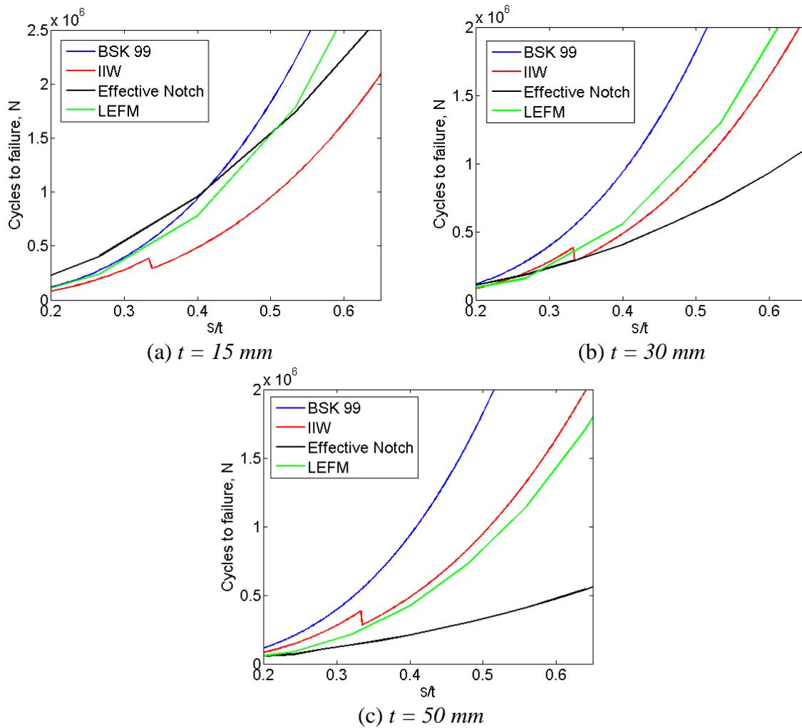
**Figure 37** Number of cycles to failure is plotted, for the four different calculation methods, against the quotient of weld throat thickness,  $s$ , and plate thickness,  $t$ . The nominal stress applied is 60 MPa. BSK 99 and IIW gives the same estimation of the lifetime for all plate thicknesses, while the lifetime decreases when the thickness is increased for effective notch and LEFM. Especially for the effective notch method, this effect is significant.
