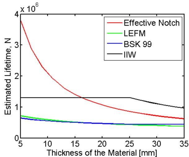
**Figure 33** The effective notch method, LEFM, BSK 99 and IIW all estimates the lifetime different. The BSK 99 and LEFM are quite similar. IIW are slightly higher and the effective notch method predicts a much longer lifetime, especially for small thicknesses.
