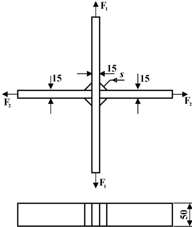
Figure 40 The cruciform joint used for fatigue tests.
