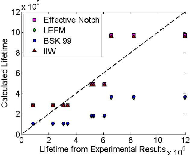
**Figure 52** Non load-carrying joint. BSK 99 and LEFM give estimations similar to each others and IIW and effective notch give approximately the same results.
