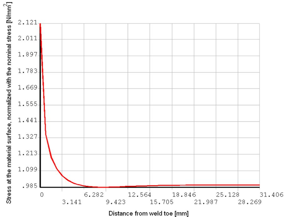
**Figure 12** The stress at the material surface decreases as the distance from the weld increases. Eventually the stress equals the nominal stress. The plate thickness is 15 mm.
