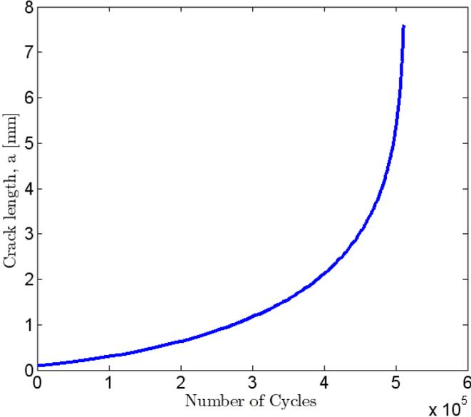
**Figure 26** The thickness of the material is *15 mm*. When the crack length approaches half the thickness (*7.5 mm*) the number of cycles required, to make the crack grow, are fewer. The lifetime left before failure is negligible.
