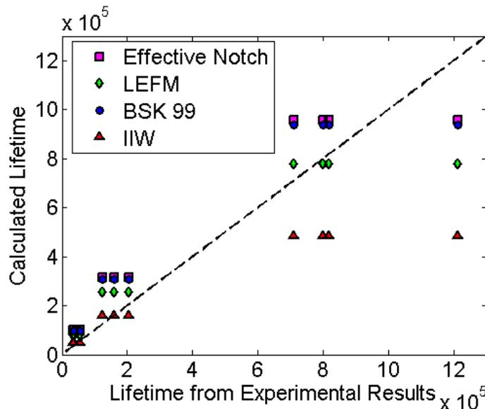
**Figure 54** Load-carrying joint with small weld size. IIW underestimates the lifetime but the other methods are quite good. Perhaps LEFM is the best method for this particular joint.
