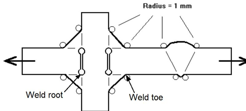
**Figure 7** In the effective notch method the notches at weld toe and weld root are fictitiously rounded. [5]
