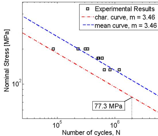
**Figure 42** Experimental results for the non load-carrying joint. The slope of the curve,  $m$ , is determined by linear regression and  $\log C$ , in equation 2:5, is determined by statistics according to the recommendations from IIW. [5]
