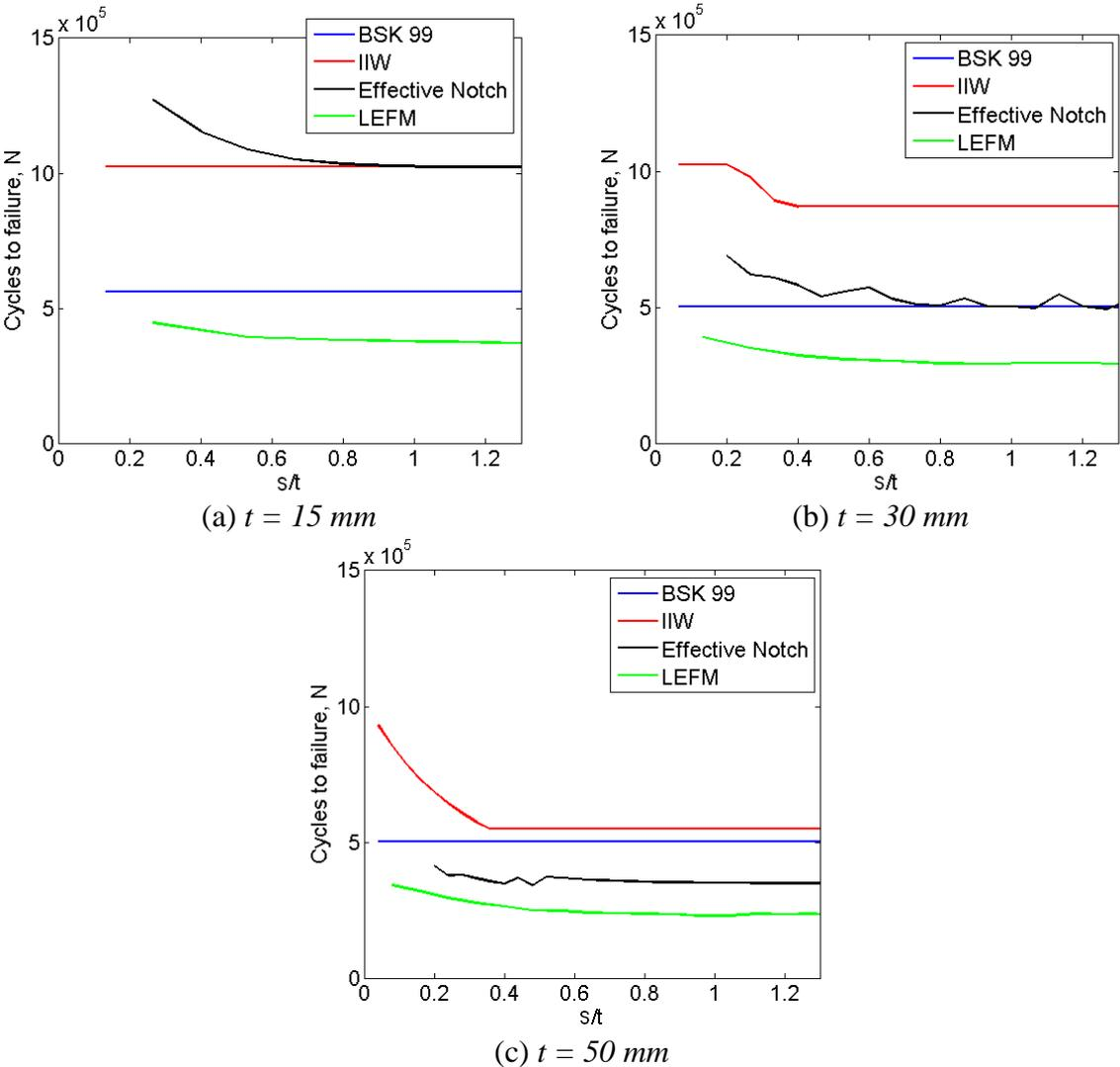
**Figure 39** For the non load-carrying joint the number of cycles to failure is plotted versus the quotient  $s/t$ . The nominal stress range applied is 130 MPa.
