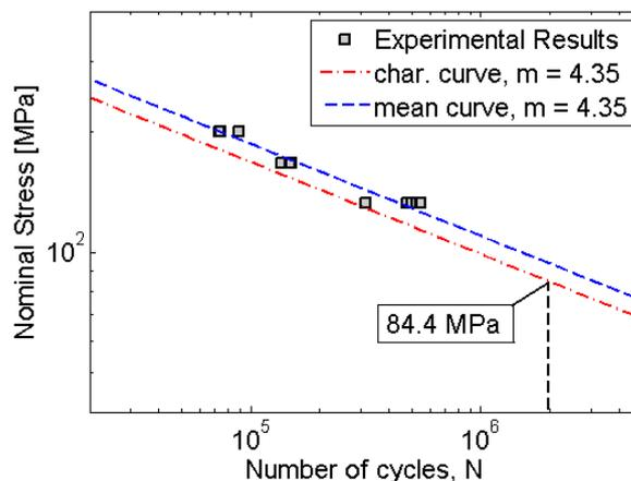
**Figure 46** Experimental results for the load-carrying cruciform joint with the big weld size. The slope,  $m$ , is determined by linear regression and  $\log C$ , in equation 2:5, is determined by statistics according to the recommendations from IIW [5].
