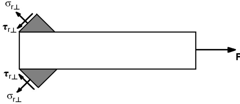
**Figure 56** The force situation in a load-carrying cruciform welded joint.
