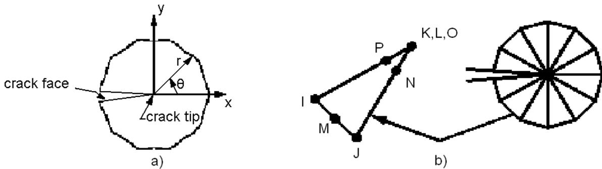
**Figure 21** In Ansys the singularity in the crack tip is modelled by skewing the midside nodes to a quarter of the distance from the tip. [13]
