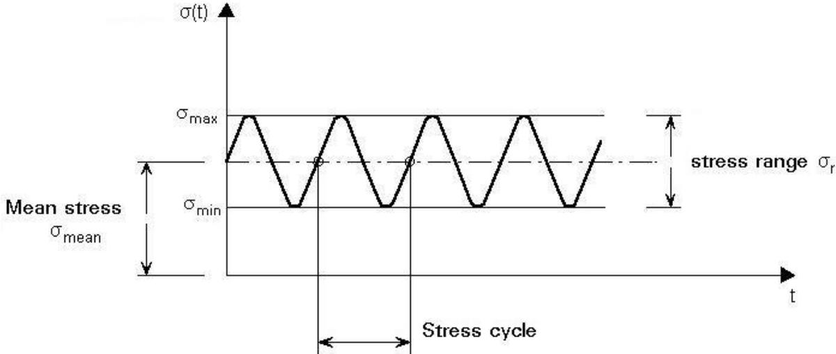
Figure 3 Fluctuating stress with constant stress amplitude and constant mean stress.
