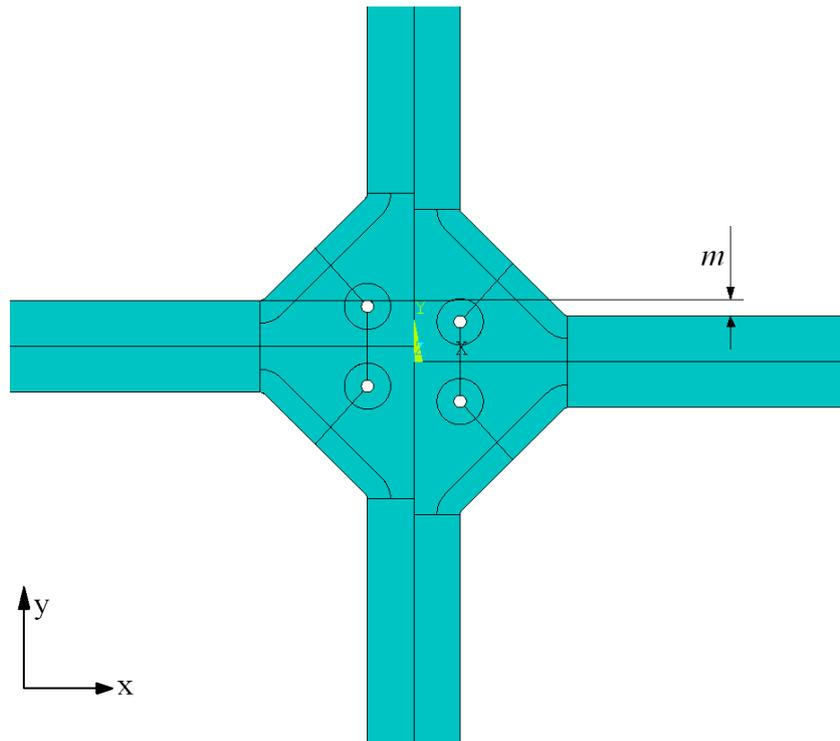
**Figure 35** An axial misalignment is added to the model to investigate how this will affect the result. This is a load-carrying cruciform joint. The steel plate thickness is here 15 mm and  $s = 12$  mm.
