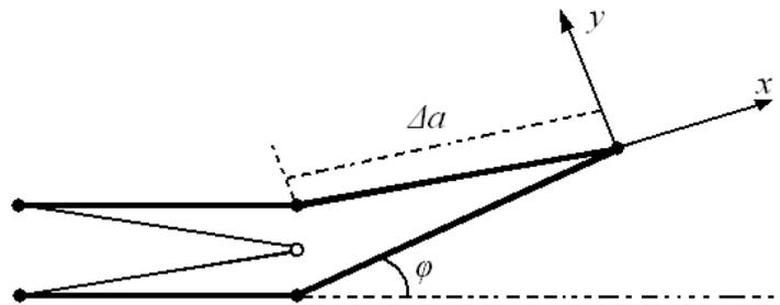
**Figure 23** The crack growth increment and the deflection angle between the crack front and the crack extension decide where the next crack tip will be placed.
