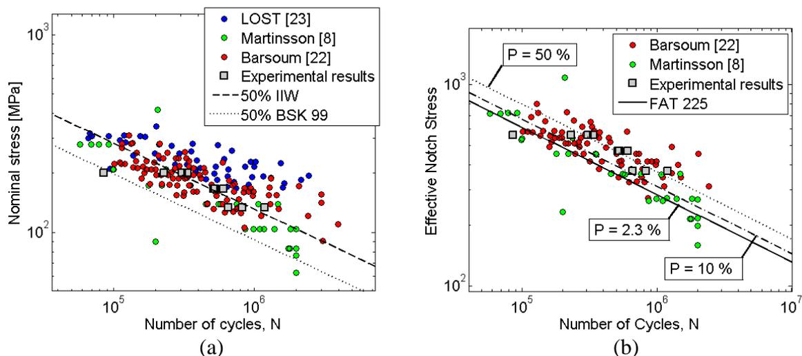
**Figure 43** The experimental results are compared to previously done fatigue tests. In (a) the nominal stress range is on the y-axis, and the curves for 50 % failure probability are plotted for IIW standard and BSK 99 standard, respectively. In (b) the effective notch stress range is on the y-axis, and the curves for different failure probabilities are included in the figure.
