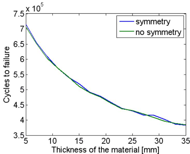
**Figure 22** There is no significant difference for the estimated lifetime when the model is made with or without symmetry.
