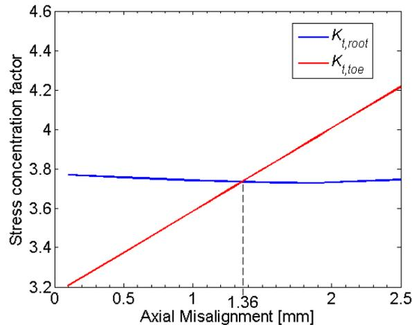
**Figure 36** A load-carrying joint, with  $t = 15$  mm and  $s = 12$  mm, is modelled with misalignment to see how this affects the relation between the stress concentration factor in the root and the factor in the toe. When the misalignment is larger than 1.36 mm, the stress concentration factor in the toe becomes larger than the one in the root.
