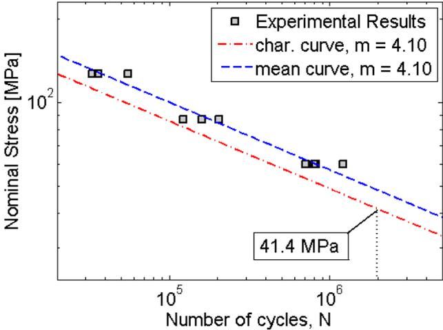
**Figure 48** Experimental results for the load-carrying cruciform joint with the small weld size. The slope, *m*, is determined by linear regression and log *C*, in equation 2:5, is determined by statistics according to the recommendations from IIW [5].
