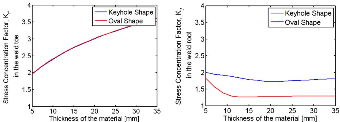
**Figure 16** The difference in the stress concentration factor when modelling with a keyhole shaped root and an oval shaped root. For the result in the weld toe there is no significant difference but for the weld root the differences are greater.
