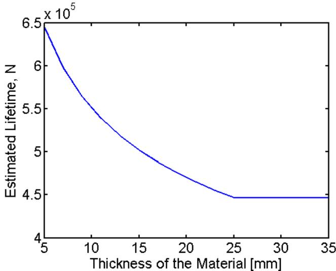
**Figure 31** For the nominal method, due to BSK 99, the thickness of the material only have effect on the lifetime when the thickness is thinner than  $25 \text{ mm}$ .
