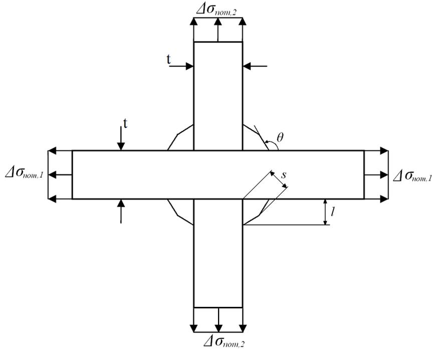
**Figure 11** The cruciform joint used for analysis.  $\Delta\sigma_{nom,1}$  gives a non load-carrying joint and  $\Delta\sigma_{nom,2}$  gives a load-carrying joint.
