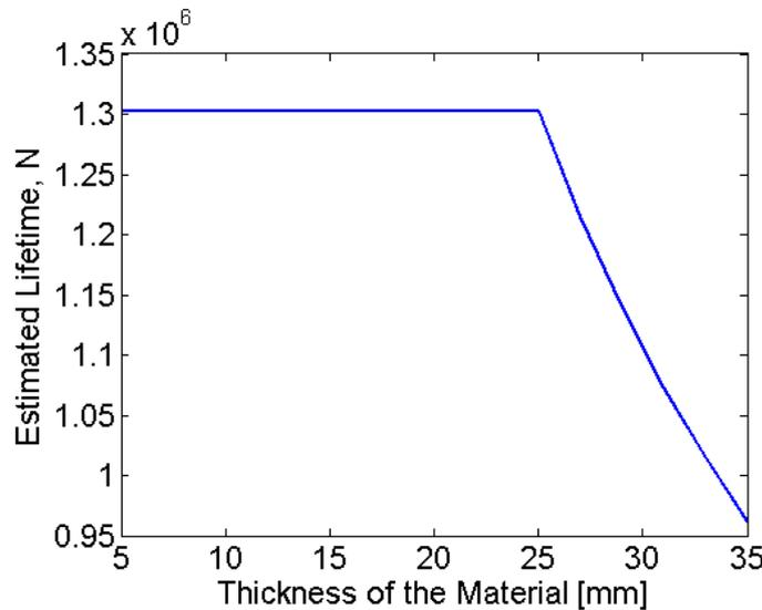
**Figure 32** For the nominal method with the standard of IIW the thickness only affects the estimated lifetime if the thickness is above 25 mm.
