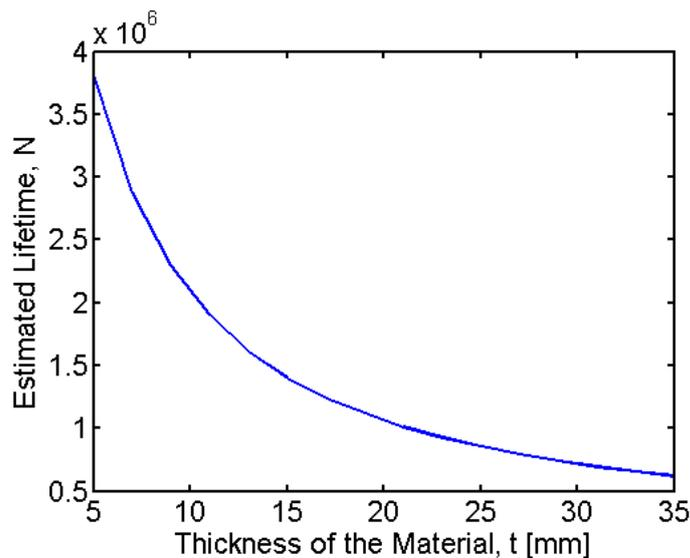
**Figure 18** Estimations of the lifetime due to the effective notch method is highly dependent on the steel plate thickness.
