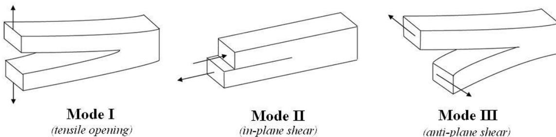
**Figure 9** A crack can be loaded in three different modes. Mode I is the most dangerous way to load a crack since this will cause the greatest stress intensity.
