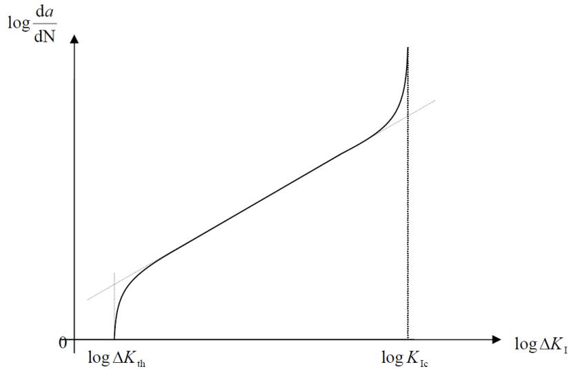
**Figure 10** The crack increment per load cycles is plotted logarithmically as a function of the stress intensity rate. Below the threshold value of the stress intensity rate,  $\Delta K_{th}$ , the crack will not propagate. Above the critical value,  $\Delta K_{Ic}$ , a fracture will occur momentarily.
