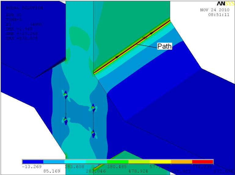
**Figure 44** The 3D modelled is made to see how a decentralized attachment in the test machine affects the result. The stress is measured along the path marked in the picture.
