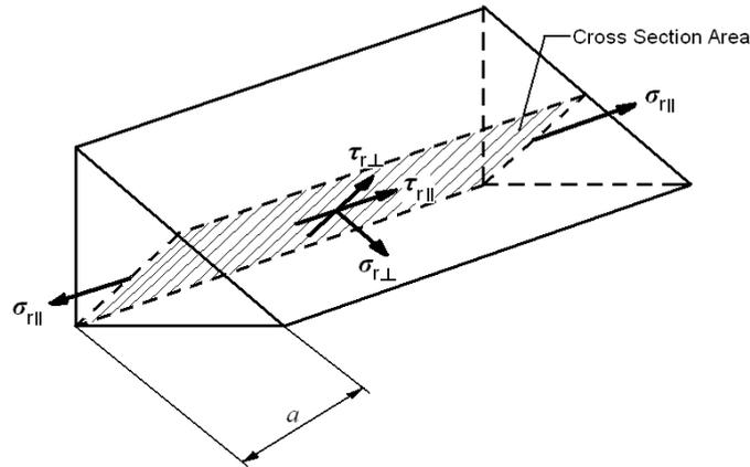
**Figure 55** The stress components in the cross section area through the fillet weld.
