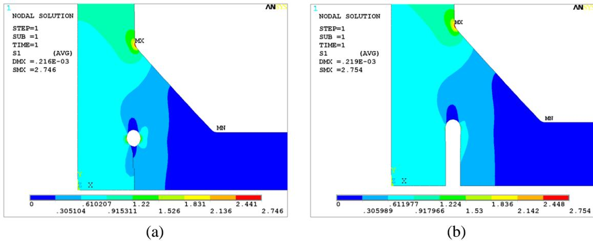
**Figure 15** The root notch is modelled with a keyhole or with an oval shape. The contour is the first principal stress.
