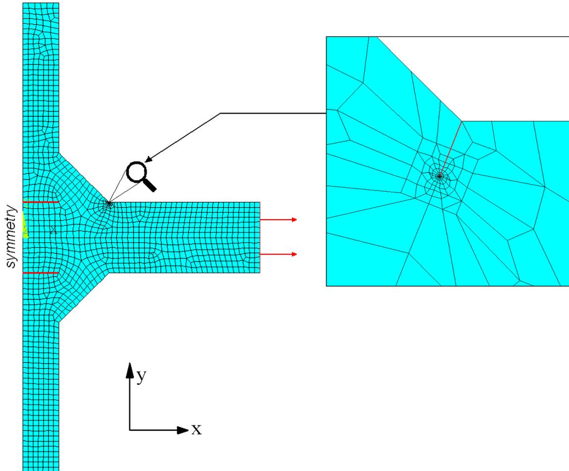
**Figure 20** With the method LEFM a single symmetry model is used. The crack is initiated perpendicular to the maximal principal stress and the elements have to be relatively small around the crack tip.
