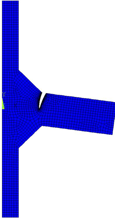
**Figure 24** For a toe crack, the crack is propagated to half the thickness of the material. In this plot the scaled deformation is showed.
