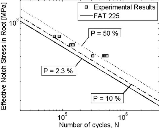
**Figure 47** The effective notch stress is plotted versus the experimental lifetime. Curves for FAT 225 are plotted for different failure probabilities. For the results to correspond to FAT 225 one of the ten dots should lie under the 10 % -curve.
