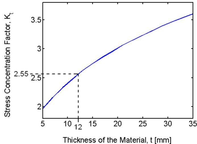
**Figure 17** The stress concentration factor increases when the material thickness increases.
