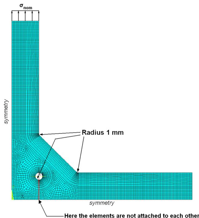
**Figure 14** The elements have to be relatively small in the radii. At least 6 elements per 90° are needed. Also in the normal direction the elements has to be rather small due to the large stress gradient in that direction. [10] [11]
