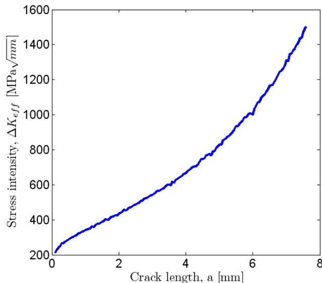
**Figure 25** The stress intensity factor increases as the crack length increases. Eventually it will reach the critical value,  $\Delta K_{IC}$ . The thickness of the material is here  $15\text{ mm}$ .
