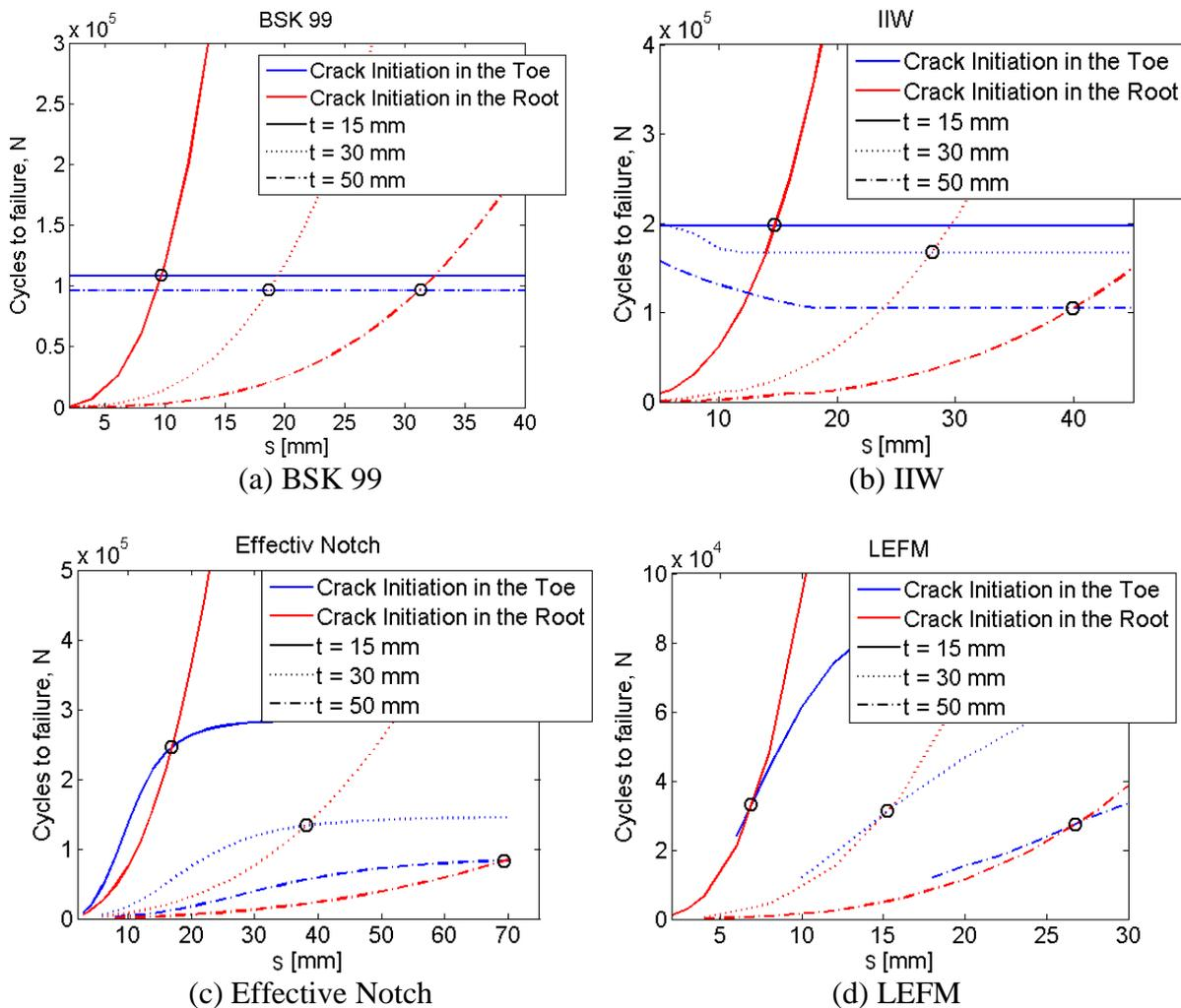
**Figure 34** For the four evaluation methods the critical value of the weld throat thickness,  $s_{critical}$  is determined for when the crack moves from a root crack to a toe crack. Blue lines are for analyses where the crack is assumed to start at the weld toe and red lines are for analyses where the crack is assumed to start at the weld root. The different dotted lines are for different plate thicknesses.
