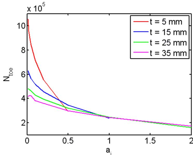
**Figure 30** The estimated lifetime vs. the length of the initiated crack in mm. The curves are steep when the initiated crack is small, indicating that much of the lifetime is consumed while the crack is small. There is a huge different in lifetime for a small and a large initial crack, especially when the material thickness is small.
