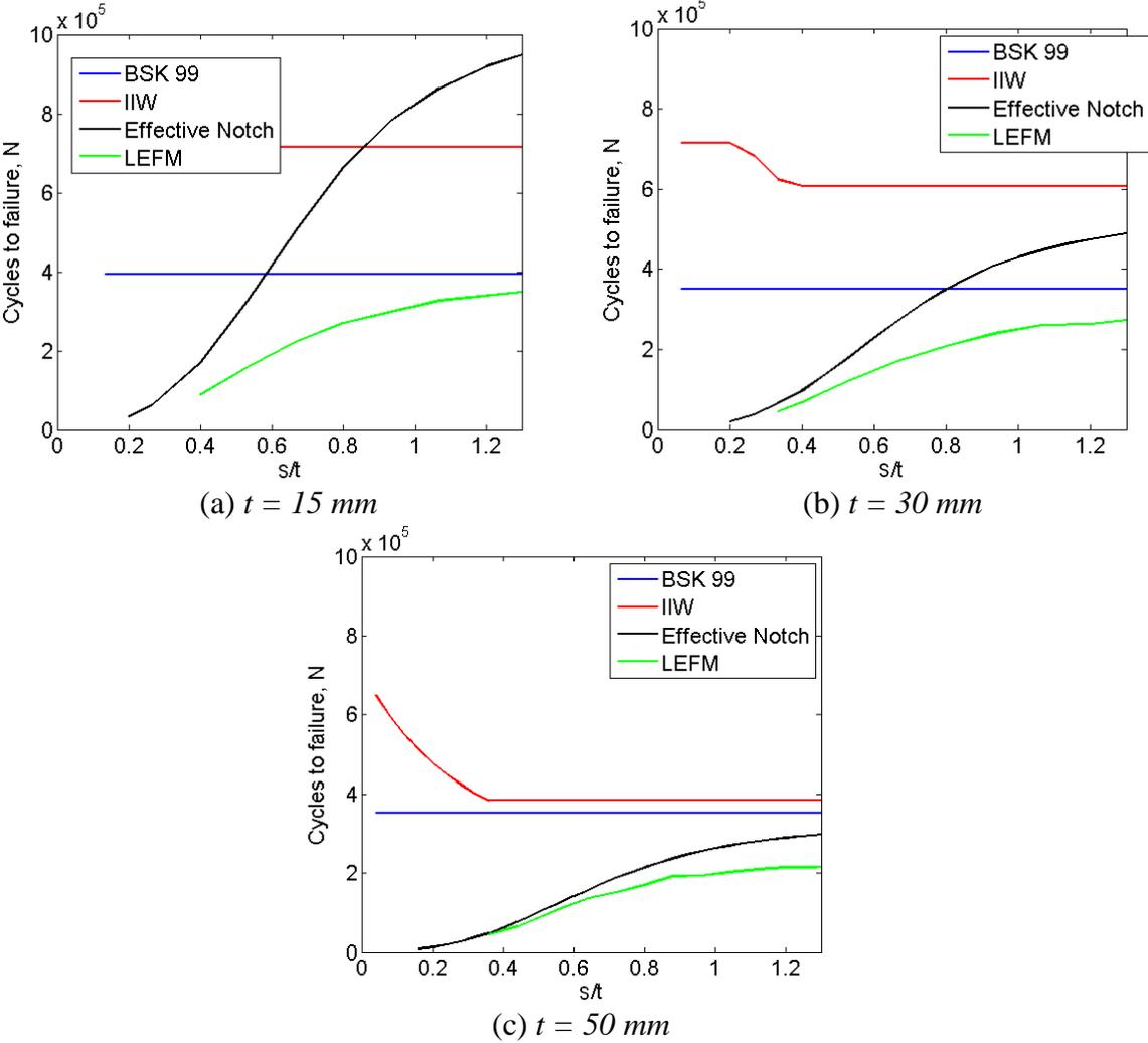
**Figure 38** The number of cycles to failure is plotted against the quotient  $a/t$  for the load-carrying joint where the crack is initiated in the weld toe. The nominal stress applied is 130 MPa. Results for  $s/t < 0.6$  is not really of interest here since then the crack would be initiated in the root.
