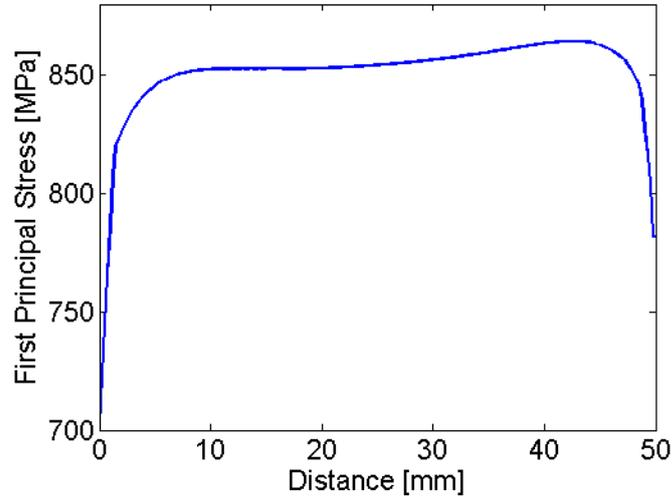
**Figure 45** The largest principal stress varies along the path in **Figure 44**. The non symmetrical difference in the stress is according to the non symmetrical fastening in the test machine. The difference is approximately 1.3 %.
