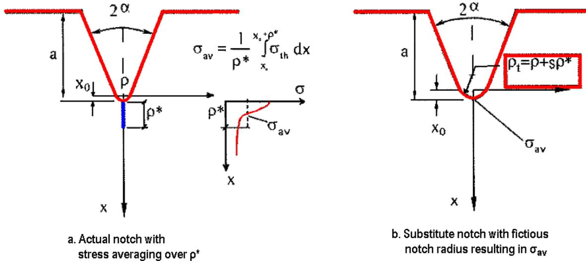
**Figure 8** The actual notch is substituted by a fictitious notch radius to obtain a stress concentration that includes the microstructural support effect. [9]
