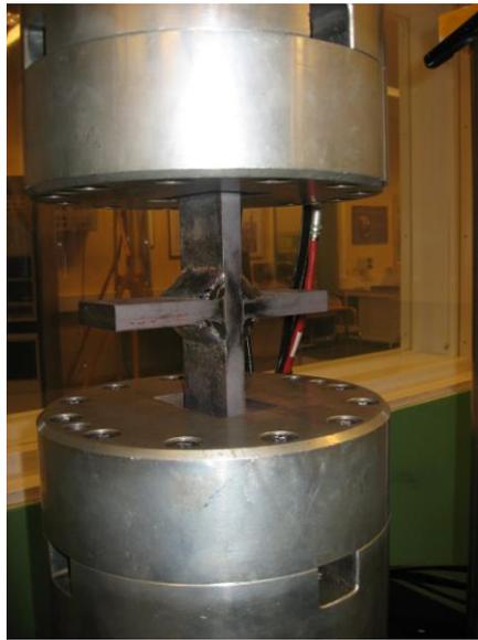
**Figure 41** *The specimen is attached to the test machine. This is a non load-carrying joint.*
