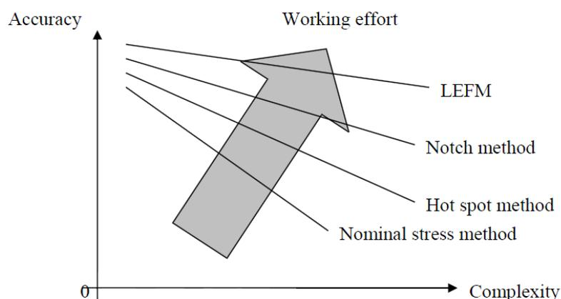
**Figure 6** There are essentially four methods for dimensioning against fatigue failure. The nominal stress method is the least complex and least time consuming one, but also the least accurate one. Linear elastic fracture mechanics is considered to be the most accurate one but at the expense of complexity and more working effort. [4]
