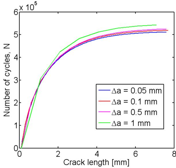
**Figure 29** For a material thickness of 15 mm the estimated lifetime decreases when the crack increment decreases. The result for the smallest crack increment should be the most accurate one.
