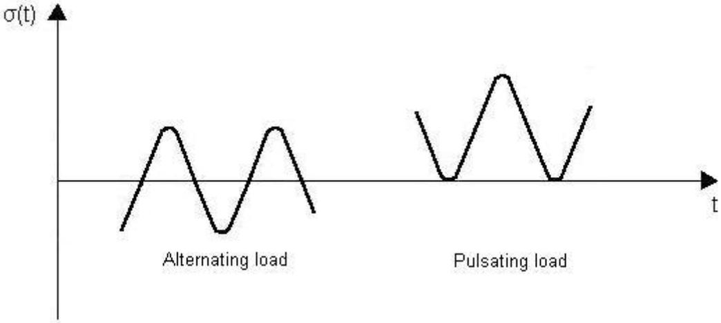
Figure 4 Alternating and pulsating loads.
