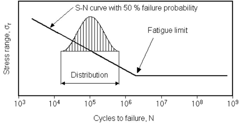
**Figure 5** Example of an S-N curve relating the stress range to the number of cycles to failure.
