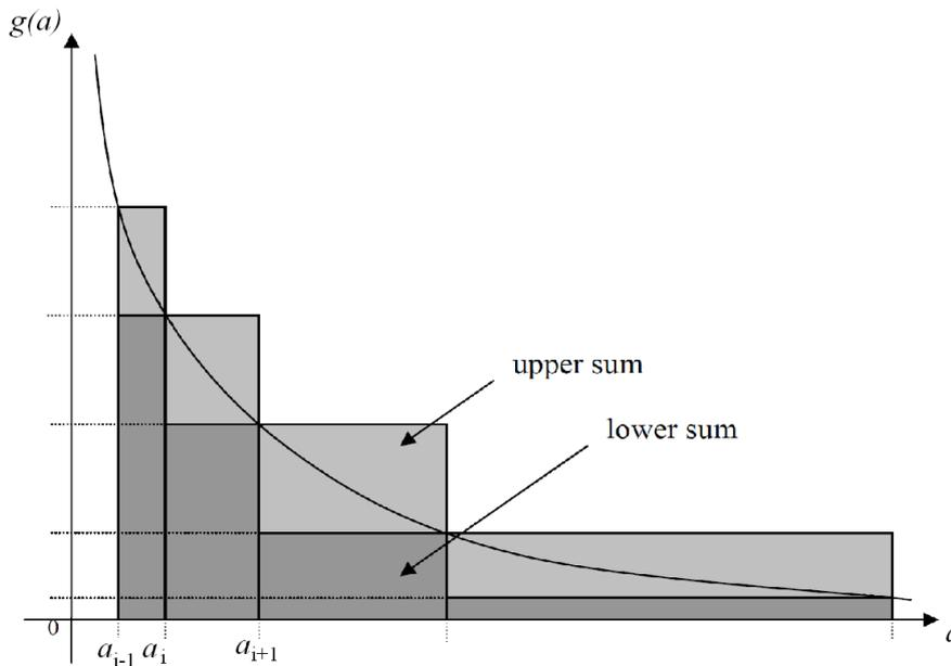
**Figure 27** A mean value of the upper and lower sum will give the most accurate result when integrating numerically.
