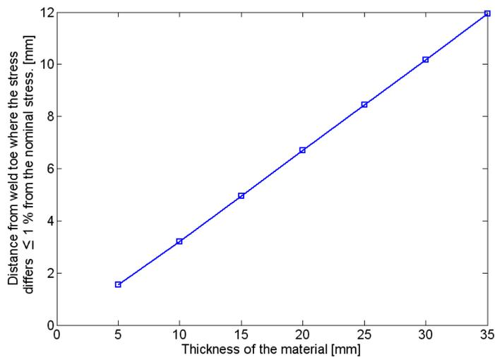
**Figure 13** The distance from the weld toe where the stress is approximately equal to the nominal stress depends linear in the thickness of the material. (Note that here,  $s=t/2$ , so the dependence is also linear in  $s$ .)
