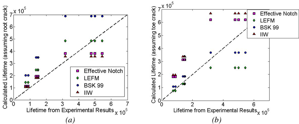
**Figure 53** Load-carrying joint with the large weld size. In (a) the calculations are based on the assumption that the crack grows from the root and in (b) that the crack grows from the toe. Effective notch and IIW are most conservative for a root crack, while LEFM and BSK 99 are predicting a toe crack.
