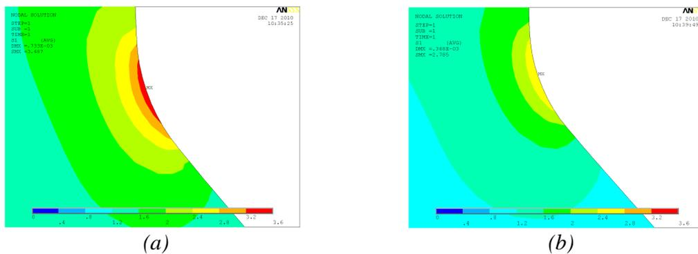
**Figure 19** The stress gradient is larger for a thicker steel plate. This decreases the fatigue resistance in the structure.
