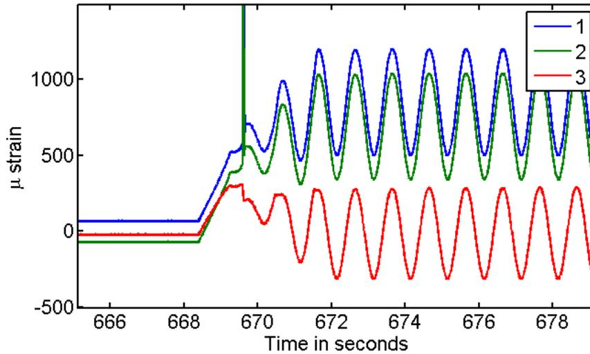
**Figure 51** For the three strain gauges the strain is measured in time. The unit on the y-axis is  $\mu$  strain (strain  $\cdot 10^{-6}$ ).
