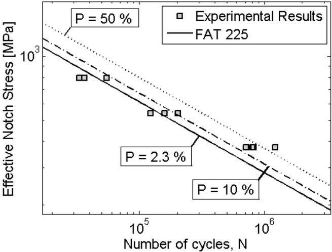
**Figure 49** The effective notch stress is plotted versus the lifetime. Curves for FAT 225 are plotted for different failure probabilities. For the FAT-value to agree with the results, one of the ten specimens should lie below the 10 % -curve and the other ones should lie above it.
