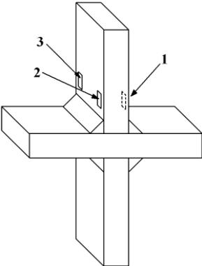
**Figure 50** Three strain gauges are attached to a test specimen in this way. They are located ca 5 mm from the edge of the steel bar.
