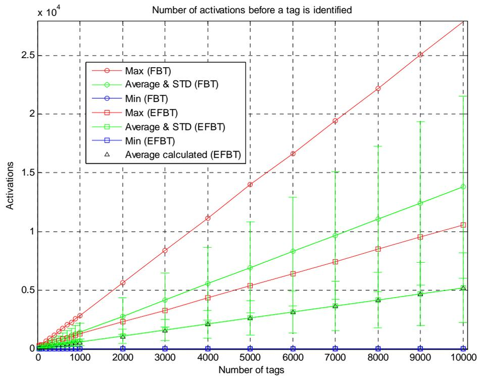
FIGURE 5. WHEN USING THE ENHANCED PROTOCOL (EFBT) THE AVERAGE NUMBER OF ACTIVATIONS WITH A POPULATION OF 1000 TAGS IS DECREASED BY 2.5 TIMES. THE MAXIMUM NUMBER OF ACTIVATIONS IS DECREASED BY 2.2 TIMES. THE CALCULATED AVERAGE FOR THE ENHANCED PROTOCOL COINCIDES WITH THE SIMULATED AVERAGE.
