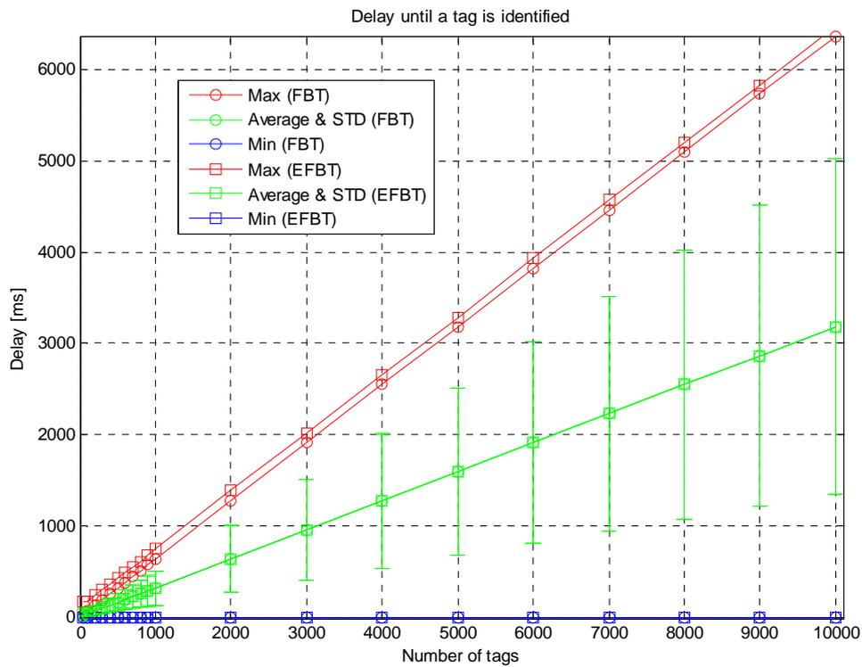
FIGURE 6. THE DELAY OF THE TWO PROTOCOLS. FOR EXAMPLE, WHEN THERE ARE 1000 TAGS AVAILABLE TO THE READER, THE ENHANCED PROTOCOL HAS AN INCREASED MAX DELAY OF 17 %, BUT THE AVERAGE DELAY WITH THE SAME NUMBER OF TAGS IS ONLY INCREASED BY 0.9 %.
