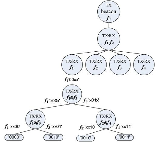
FIGURE 3. STRUCTURE OF THE FREQUENCY BINARY TREE. THE READER INITIATES A READING WITH THE BEACON (TOP LEVEL). THEN IT CHECKS WHAT FREQUENCIES F1-F4 TAGS ARE RESPONDING AT (2ND LEVEL) AND, IN THE 3RD LEVEL, IT RANDOMLY CHOOSES ONE OF THOSE AND TRANSMITS ON THAT FREQUENCY, IN THIS CASE ON F1. IN THE FOLLOWING STEPS IT RANDOMLY CHOOSES A FREQUENCY TO CONTINUE WITH UNTIL IT REACHES THE END AND HAS READ THE ID(S).
