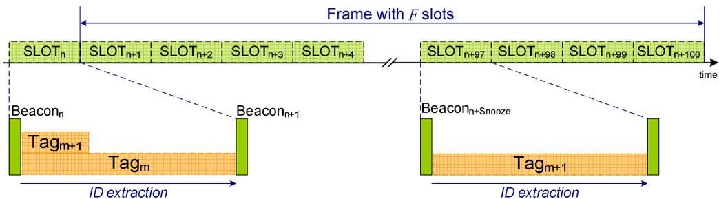
FIGURE 4. AFTER Beacon<sub>n</sub>, Tag<sub>m+1</sub> CONTENTS WITH Tag<sub>m</sub> TO DELIVER ITS ID. Tag<sub>m+1</sub> IS NOT SELECTED BY THE READER AND RANDOMLY CHOOSES A NEW SLOT IN A NEW FRAME WITH  $F$  SLOTS ( $F=100$ ) TO WAKE UP IN. IT SNOOZES UNTIL THE CHOSEN SLOT ARRIVES, AND ONCE AGAIN IT TRIES TO DELIVER ITS ID AND SUCCEEDS.
