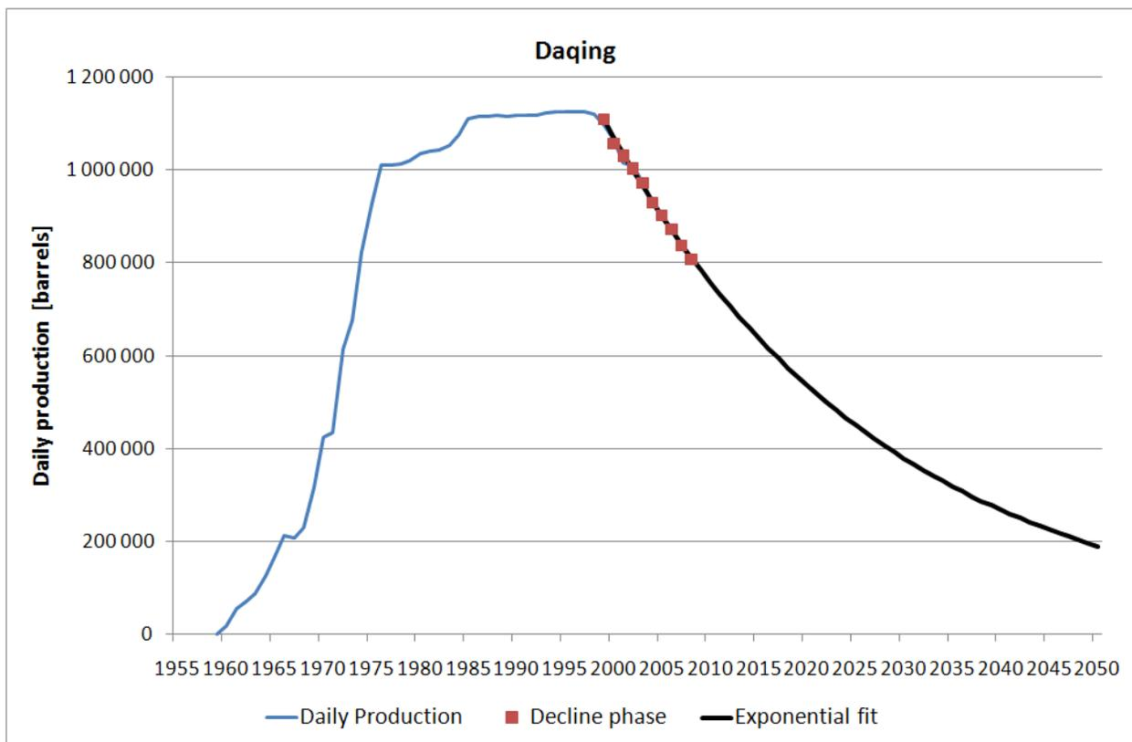
**Figure 3:** Production outlook for the Daqing oil field. The hyperbolic case is the same as the exponential case and is omitted. Daqing will remain an important oil producer for many decades, but is expected to be delivering around 200 000 b/d in 40 years.
