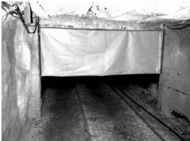
Figure 11. Brattice blockage of smoke /34/.
