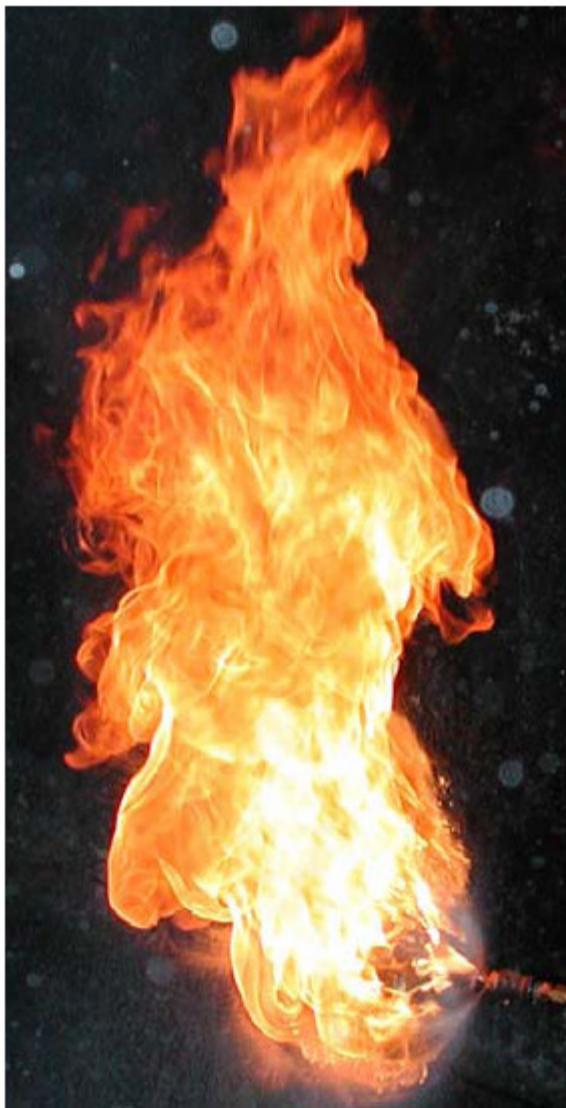
Figure 3. A hydraulic fluid spray fire /6/.
