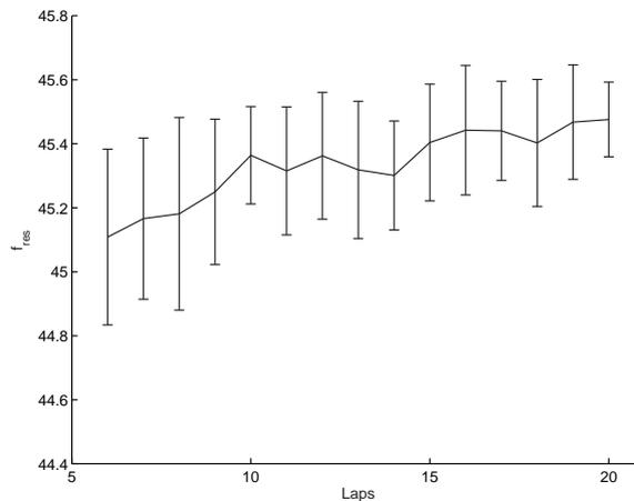
Figure 2: Resonance frequency  $f_{res}$  in Hertz versus batch size in number of tire laps. Bars indicates one standard deviation.
