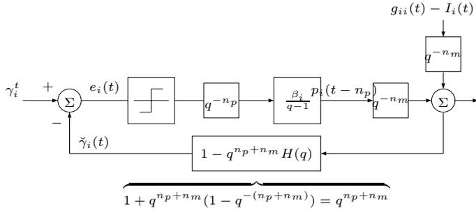
**Figure 3.** By rewriting the diagram in Figure 2, it is evident how TDC cancels the round-trip delays in the control loop. External signals and disturbances are still delayed before they are reflected in  $\gamma(t)$ .
