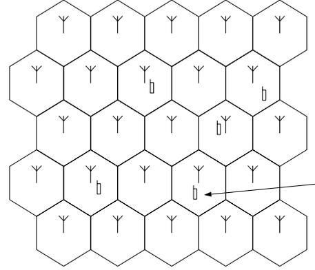
**Figure 4. Configuration in the simulation example, where four mobile stations initially are allocated to the same channel. At time instant  $t = 0$  a fifth mobile station (indicated by the arrow) is allocated to the channel.**
