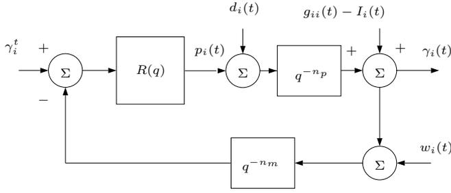
**Figure 1. The local loop dynamics when employing the general linear control algorithm  $R(q)$ . The measurements are subject to additive errors  $w_i(t)$ , and the output powers by quantization noise  $d_i(t)$ .**
