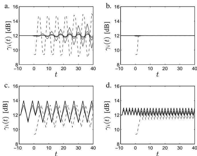
**Figure 5. The recovering ability of a. DPC, b. DPC with TDC, c. FSPC, and d. FSPC with TDC, when subject to the situation in Figure 4 and a time delay of one sample.**
