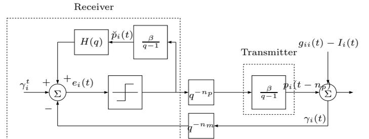
**Figure 2. Time delay compensation (TDC) can be implemented as an internal feedback by monitoring the powers to be used by the transmitter,  $\check{p}_i(t)$ . The feedback transfer function  $H(q) = 1 - q^{-(n_p+n_m)}$  is obtained from Algorithm 1i.**
