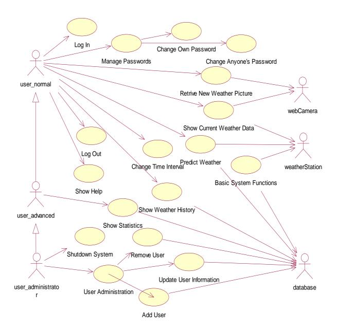
Figure 1 The use case diagram for the weather station system
