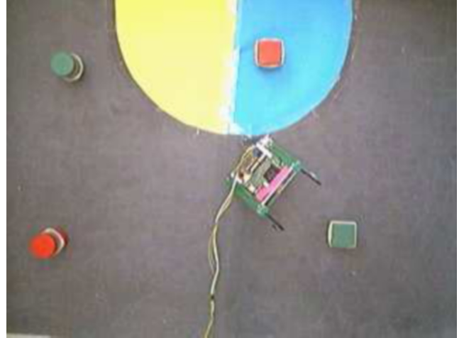
Figure 6. Example image from top mounted camera. A pink tape has been placed on the Khepera gripper to facilitate recognition of the robot's position and orientation.
