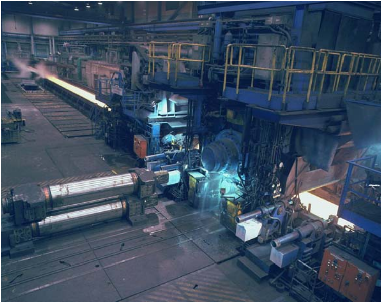
Figure 5: Steckel type hot strip finishing mill at Outokumpu Stainless Avesta works. Replacement roll pair is ready to be shifted in.
