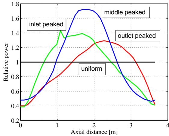
FIGURE 3.2. The four axial power distributions used in the experiments. The spike in the inlet peaked distribution is a manufacturing fault.
