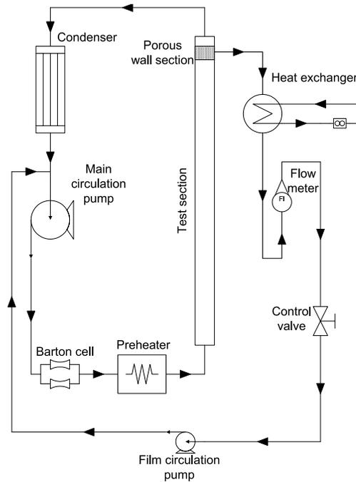
FIGURE 3.1. Working principles of the main loop and the film extraction loop.
