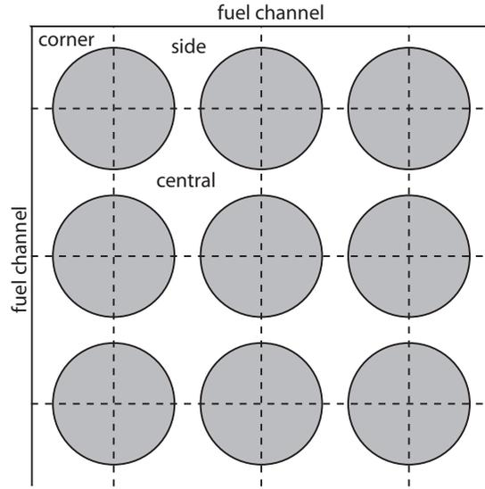
FIGURE 5.2. Typical subchannel decomposition in part of a BWR fuel bundle. Three distinct subchannel geometries arise: central, side and corner.
