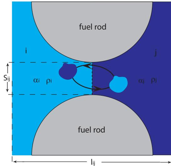
FIGURE 5.3. Idealized view of turbulent mixing in the gap between two subchannels. Fluid 'globs' of equal volume are exchanged; a density gradient between the subchannels will cause a net mass flow down the gradient.
