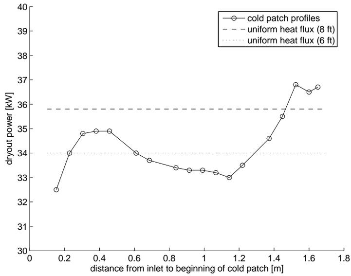
FIGURE 2.2. Experimental dryout power in 8 ft pipe with 2 ft cold patch (Bennett *et al.* 1966). Mass flux = 297 kg/m<sup>2</sup>s and pressure = 0.38 MPa.
