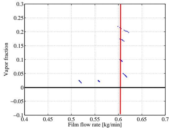
FIGURE 3.3. Example of suction curve from the experiments. The film flow rate is determined from the intersection of the vertical part of the curve with the horizontal axis.
