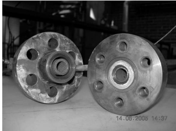
FIGURE 3.5. The porous sinter metal part mounted in the film extraction device.
