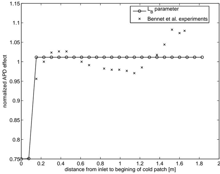
FIGURE 4.1. Relative dryout power and boiling length in experiments by Bennett *et al.* (1966)
