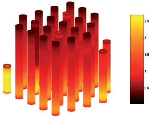
FIGURE 5.1. Three dimensional power distribution. Part-length fuel rods are visible.
