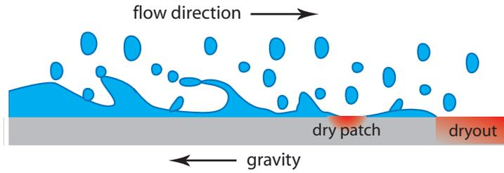
FIGURE 2.1. Idealized picture of annular flow close to a heated wall.
