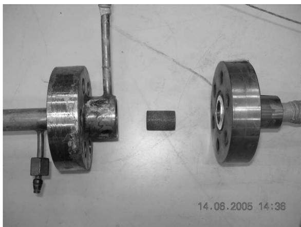
FIGURE 3.4. Side view of dismantled film extraction device.
