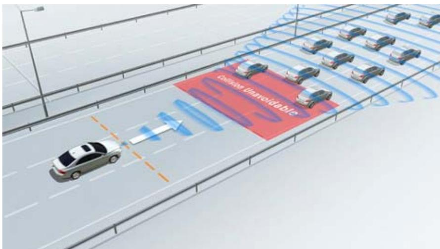
The picture shows the system functionality of the Forward Collision Warning system. ([www.media.volvocars.com](http://www.media.volvocars.com))
