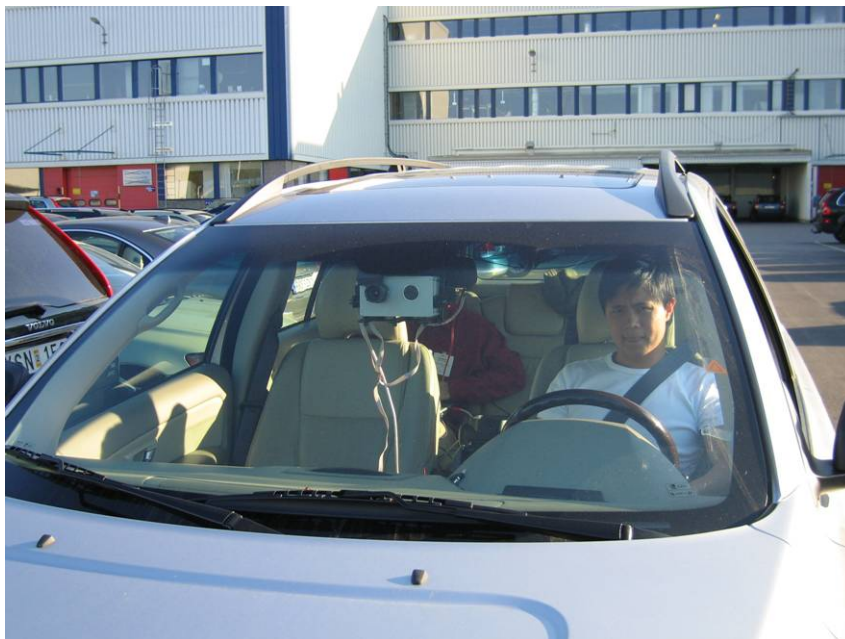
Figure 39: The Locust sensor system mounted in the XC90, seen from the outside.
