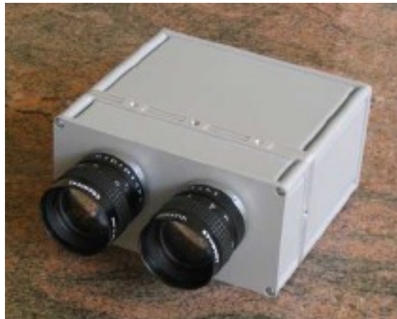
Figure 6: The Locust sensor system consists of a Bi-i unit, which holds the Locust sensor chip.
