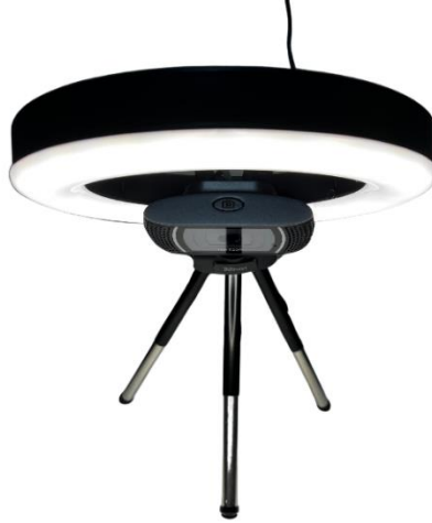
Figure 9. The setup used to detect and classify cashews with the support of a ring light.
