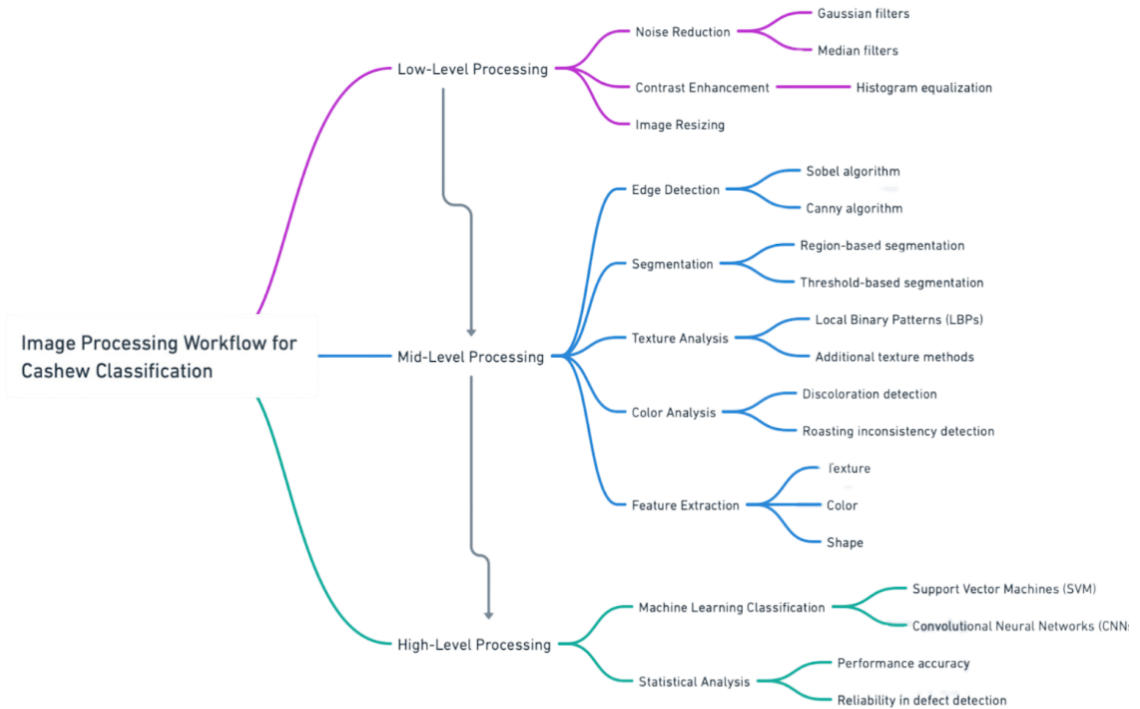
Figure 2. Illustration of the different image processing techniques at different levels
