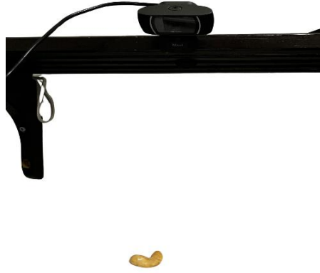
Figure 7. The setup used to detect and classify cashews in room lighting
