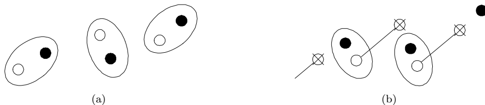
Figure 3.3. Sensor tracks are associated with each other. Figure 3.3(a) shows the case if no bias error is estimated and the two closest tracks are associated with each other. Figure 3.3(b) describes the situation when a bias error is estimated and compensated for before association is performed. Different solutions appear depending on if there is a bias error present or not.
