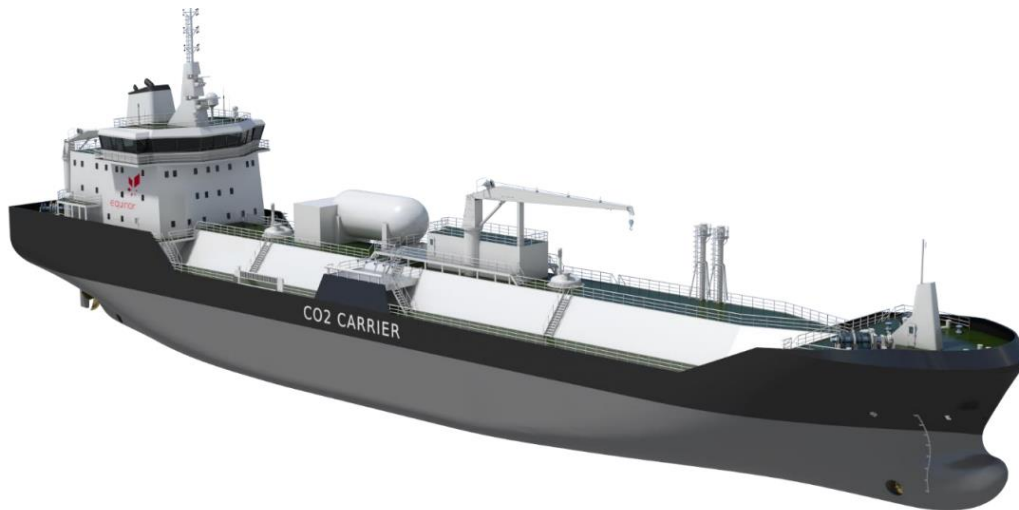
Figure 7: Liquefied CO 2 carrier tanker [57]
