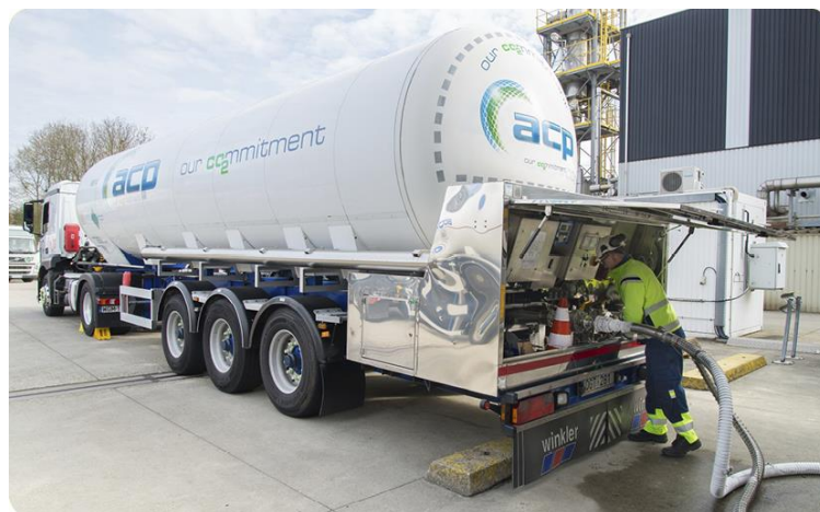
Figure 2: Loading of truck carrying liquid CO 2 [48]
