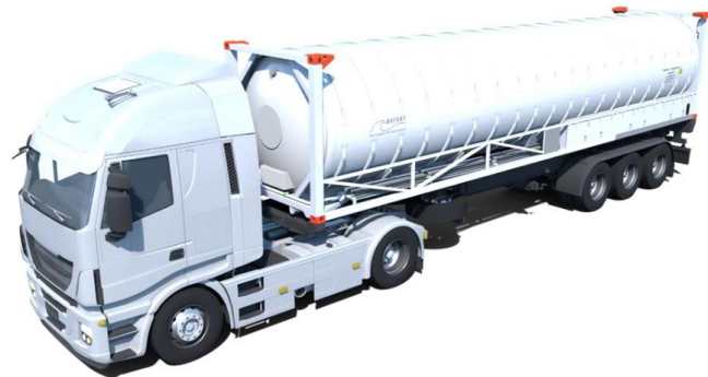
Figure 3: 40-foot tank container carried by a truck [49]
