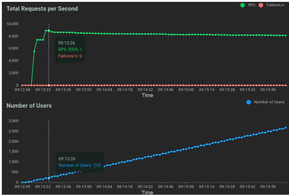
Figure 5.4: Scalability test results for the SOAP microservice. The gray dotted vertical line highlights the saturation point.
