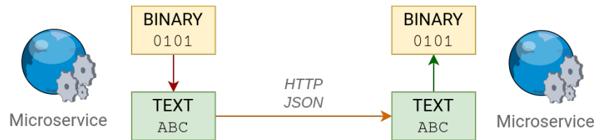
Figure 2.7: REST applications have to convert binary data to textual representation, send it over HTTP/1.x, then the receiving entity parses the text and finally converts it back to binary format.
