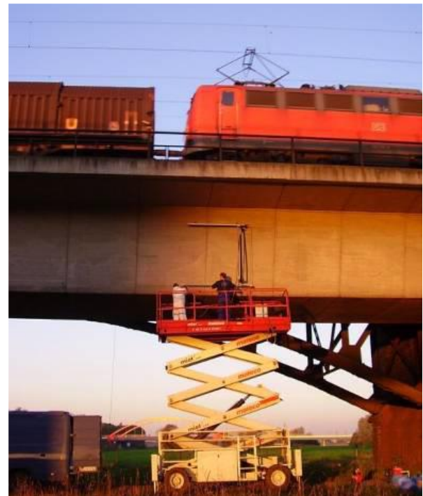
Figure 2. Automated ultrasonic scanning of a RC railway bridge in Germany (Picture: BAM)
