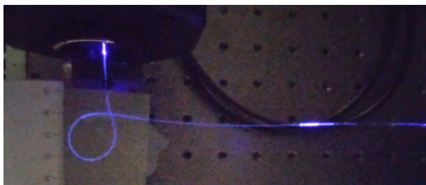
Fig. 7. Test of bending losses of a scintillating liquid-filled fiber.
