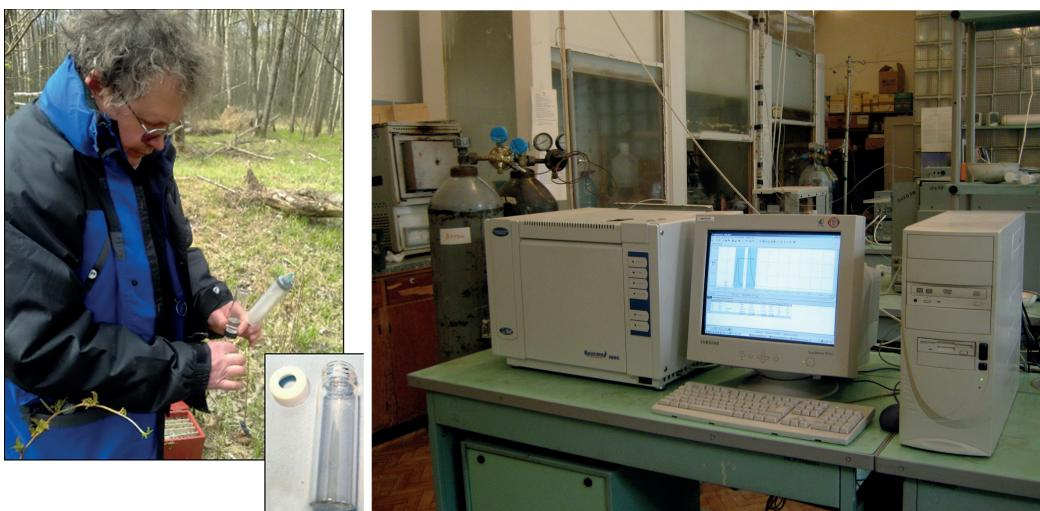
Fig. 4.3. Gas samples selection in vials for control measurements of hydrogen on chromatographs
