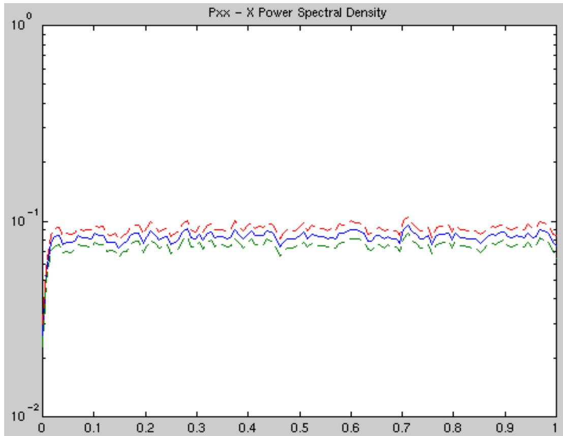
**Figure 37** Power spectral density for the random part of the Call-ID header field value. The almost constant value shows that the values are random.
