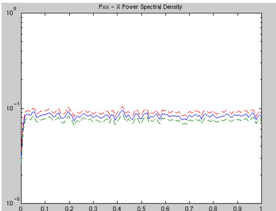
**Figure 34** Power spectral density for the random part of the Call-ID header field value. The almost constant value shows that the values are random.
