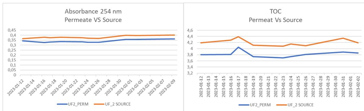
**Figure 9:** The figure to the left shows the absorbance measurements between 2023-01-12 to 2023-02-09 on source and permeate water from the ultrafiltration pilot plant. The figure to the right shows the TOC measurements between 2023-01-12 to 2023-02-02 on source and permeate water from the ultrafiltration pilot plant.
