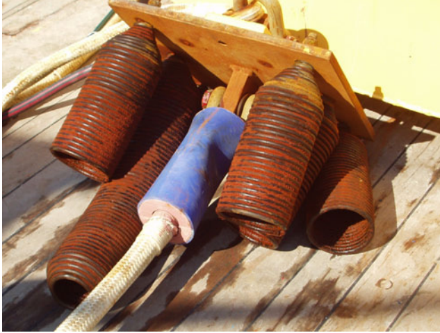
Figure 4.5: A pack of heavily corroded steel springs after having been used in force measurements during one of the earliest experiments at the Lysekil research site. The springs were placed openly and without cathodic protection in the corrosive sea water.
