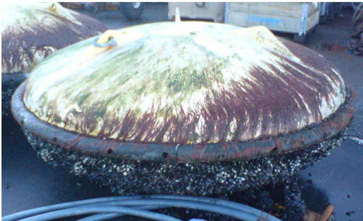
Figure 4.13: Example of biofouling on one of the biology buoys at the Lysekil wave energy research site.
