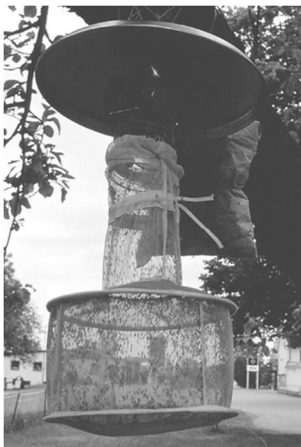
*Figure 2.* CDC miniature light trap with dry ice as an attractant (in the paper bag behind the trap). In the net some captured mosquitoes can be seen. This trap is positioned in Österfärnebo, Central Sweden. Photo by JO Lundström.
