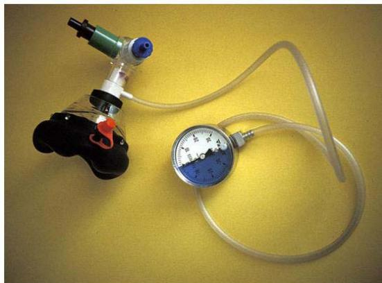
*Figure 1.* A blow bottle device and a positive expiratory pressure/respiratory muscle training (PEP/RMT) mask (Astra Tech AB, Mölndal, Sweden).
