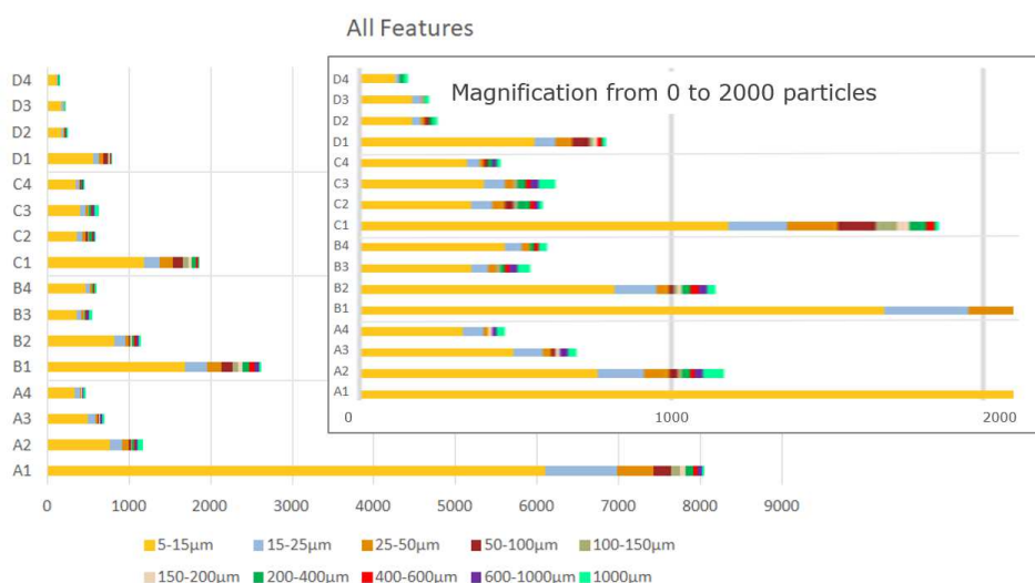
Figure 8 The results from the microscopic particle counting shows the numbers of particles (x-axis) and their size-fractions in the outlet water from the washing trials. A1 to A4 is the amount of fibre shaped particles and non-fibre shaped particles in total after washing cycles 1 to 4 when no filter was used. B1-4, C1-4 and D1-4 are results from the trials with the three different filters.
