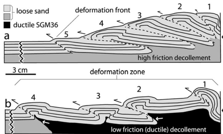
Figure 3. Line drawings of profiles of two models shortened above (a) frictional and (b) ductile décollements. Deformation zone is concentrated along the active thrust at the front of the wedge in (a) whereas in (b) the entire wedge is active.
