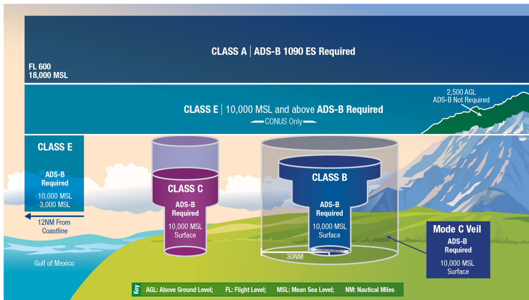
Figure 2.2: Current requirements for an ADS-B OUT transmitter in US airspace, according to the FAA [18].
