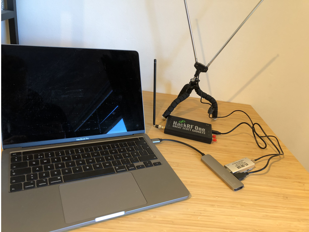
Figure 3.1: Setup used to send ADS-B messages using the HackRF One transmitter, and the RTL-SDR dongle combined with an antenna to receive the same messages.
