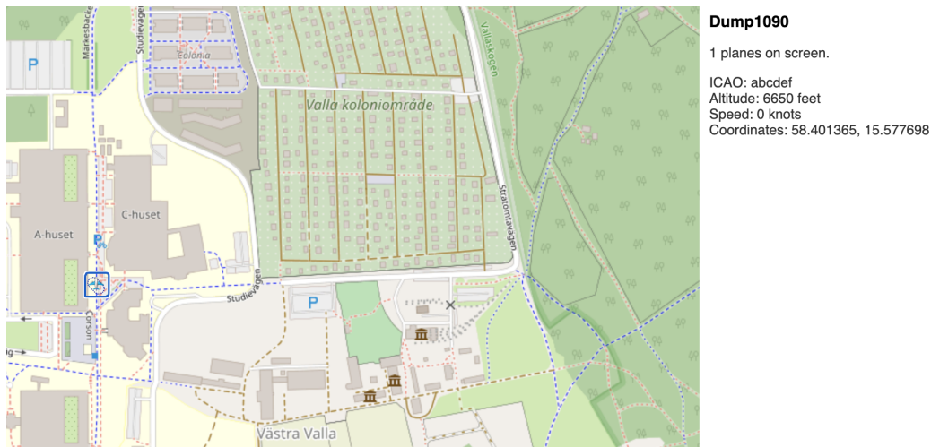
Figure 4.2: Using dump1090 with the -net flag allows the user visualize the aircraft within the web browser as well.
