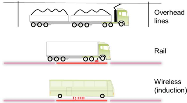
Fig. 1 The three main concepts for road electrification and power transfer to moving vehicles.
