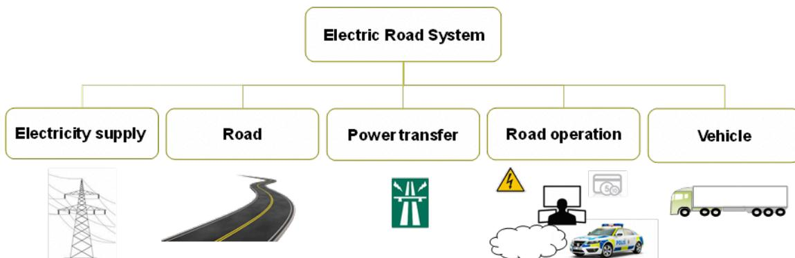
Fig. 2 Overall system layout of ERS with five subsystems.
