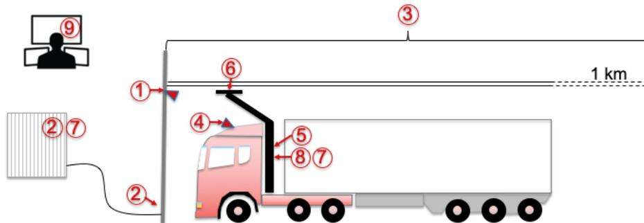
Fig. 4 Mapping of the power transfer subsystem technology elements to the Swedish demonstration project with an overhead-line solution. A energy meter (7) can be installed at different locations depending on the solution.
