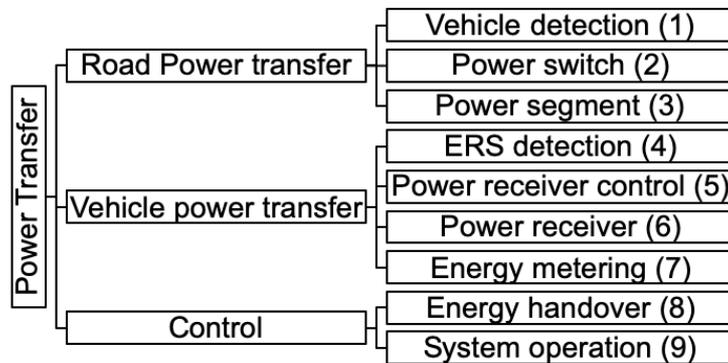
Fig. 3 Generic view of the power transfer subsystem.
