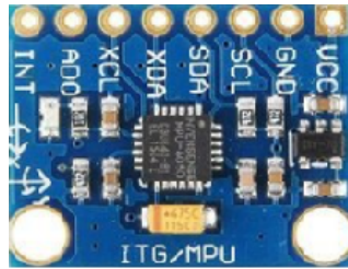
Figure 2.3: The chosen IMU for the project, model MPU6050[12]
